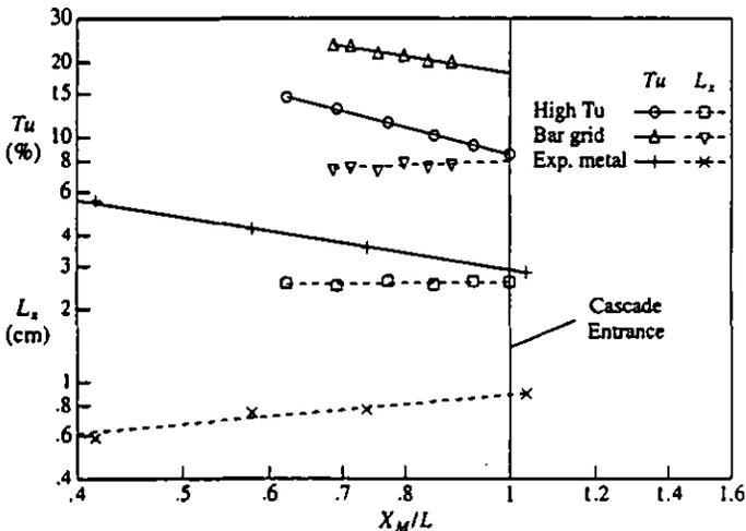
Figure 6: Decay/Growth of turbulence/scales of different turbulence generators.
