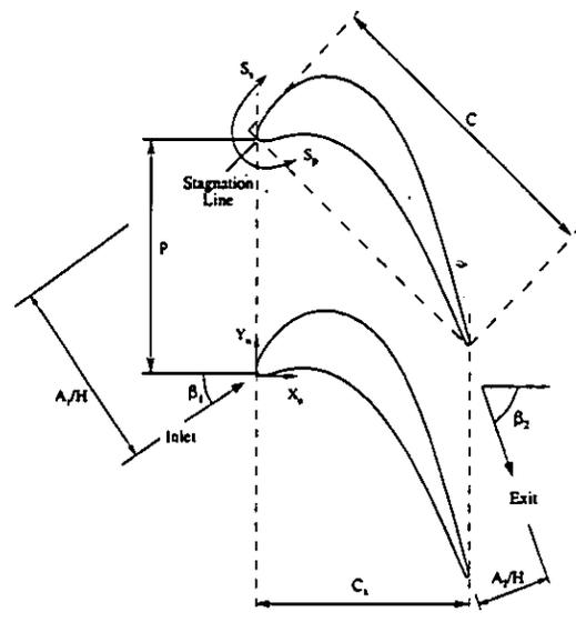
Figure 2: Central passage of the cascade and dimensions.
