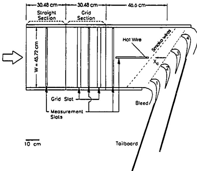
Figure 1: Schematic top view of the test section.
