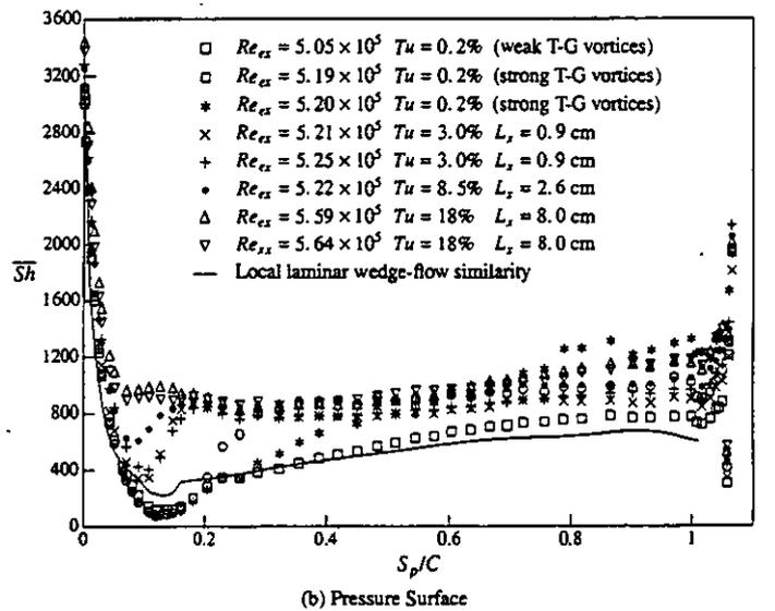
Figure 8: Sherwood number distribution for elevated turbulence levels at  $Re_{ex} = 3.6 \times 10^5$ .
