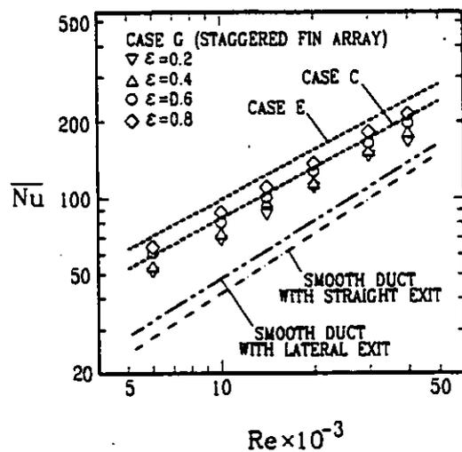
Figure 6 Reynolds number dependence of log-mean averaged Nusselt number for case G.
