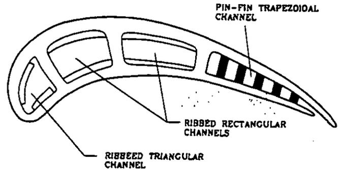
Figure 1 Cross-sectional view of the modern internally cooled turbine blade.
