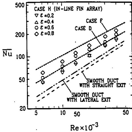
Figure 7 Reynolds number dependence of log-mean averaged Nusselt number for case H.
