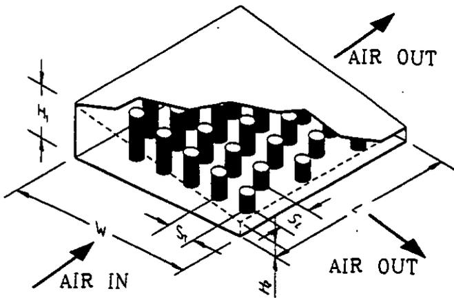
Figure 3 (a) Dimensions of the pin-fin trapezoidal duct investigated.
