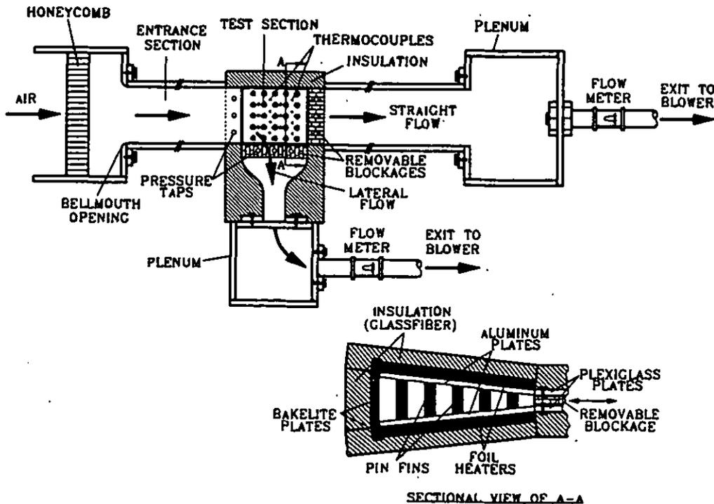
Figure 2 Sketch of the experimental apparatus, and the construction of the test section.
