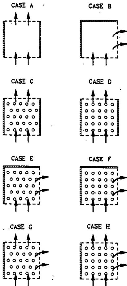
Figure 3 (b) Schematic of top view of pin-fin channels from cases A to H.
