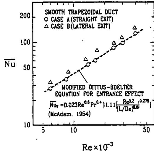
Figure 4 Comparison of average heat transfer of the present smooth trapezoidal duct and the previous correlation.
