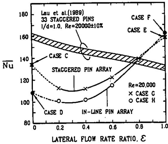
Figure 8 Effect of the ratio of lateral-to-total flow rate on log-mean averaged Nusselt number for staggered and in-line pin arrays.
