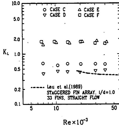
Figure 10 Reynolds number dependence of overall pressure-drop coefficient of the present pin-fin trapezoidal ducts for cases C to F.
