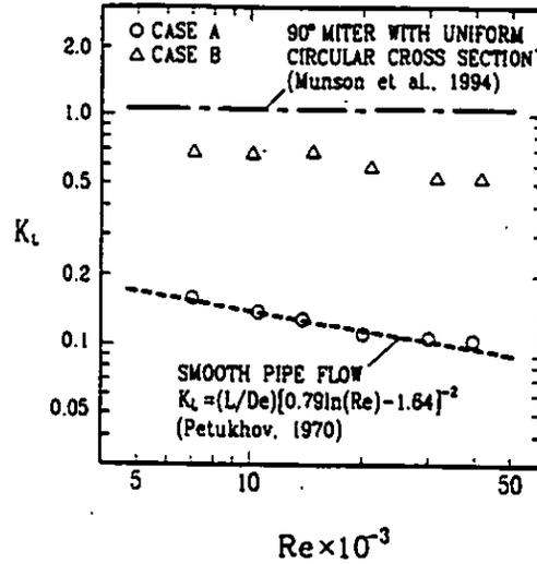
Figure 9 Comparison of overall friction coefficient present smooth trapezoidal ducts with previous correlation.
