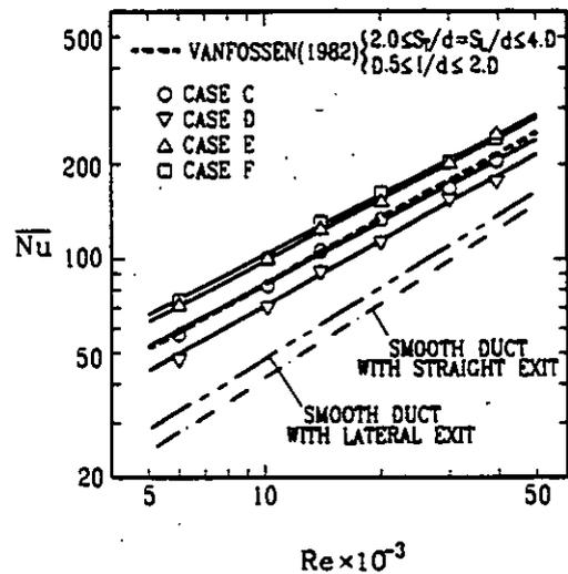
Figure 5 Reynolds number dependence of log-mean averaged Nusselt number for cases C to F.
