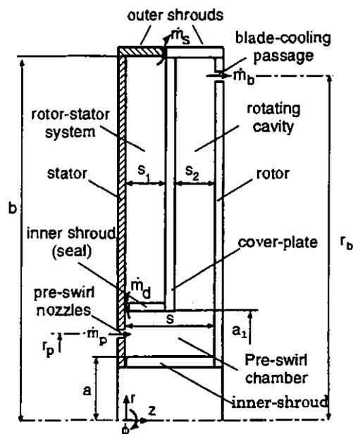
Fig 1 Simplified diagram of cover-plate pre-swirl system
