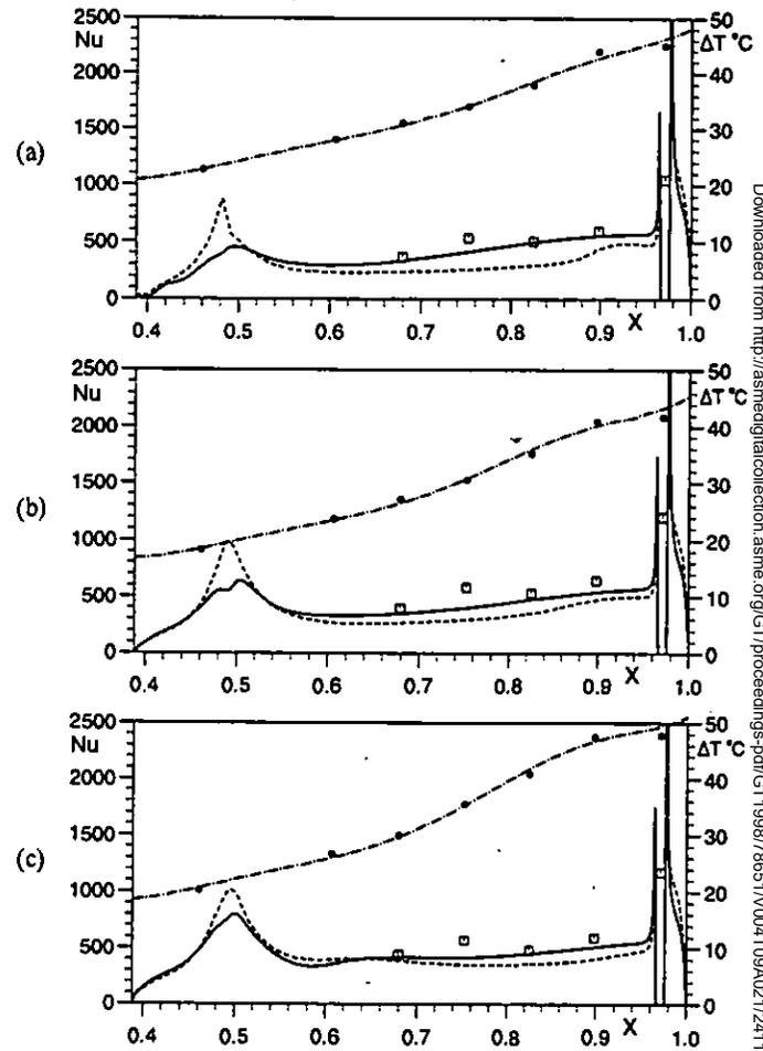
Fig 7 Comparison between computed and measured Nusselt numbers for  $Re_\phi \approx 0.5 \times 10^6$  and  $\lambda_{T,b} \approx 0.17$
