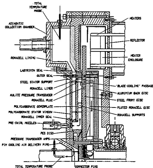
Fig 3 Details of rotating-disc rig
