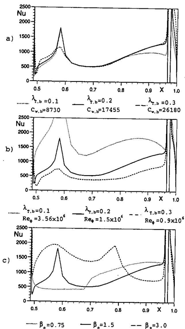
Fig 5 Computed Nusselt numbers in simple cavity
