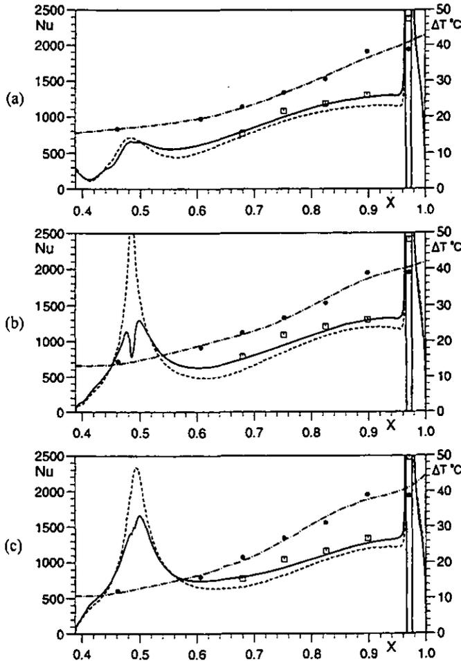
Fig 8 Comparison between computed and measured Nusselt numbers for  $Re_\phi \cong 1.5 \times 10^6$  and  $\lambda_{T,b} \cong 0.17$  (For legend, see Fig 7)
