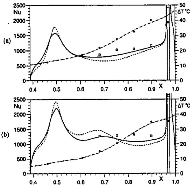
Fig 10 Comparison between computed and measured Nusselt numbers for  $Re_\phi \approx 1.2 \times 10^6$  and  $\lambda_{T,b} \approx 0.35$  (For legend, see Fig 7)
