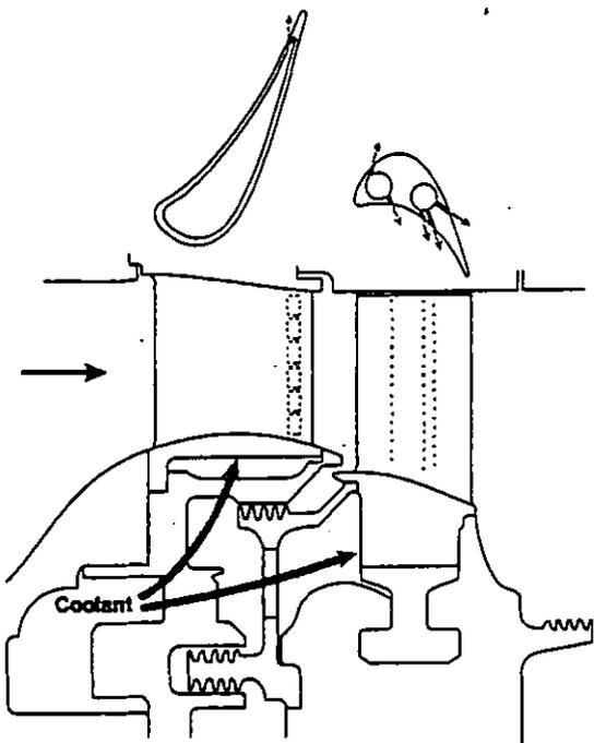
Fig. 1 ACE turbine geometry and cooling arrangement
