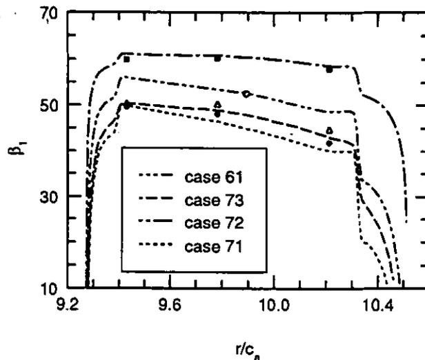
Fig. 4 Relative flow angle at rotor inlet as a function of spanwise location
