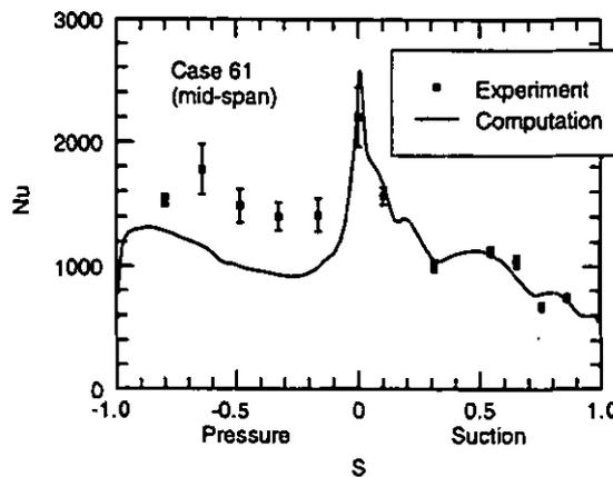
Fig. 5 Comparison of Nusselt number on the blade surface for uncooled case 61 near mid-span
