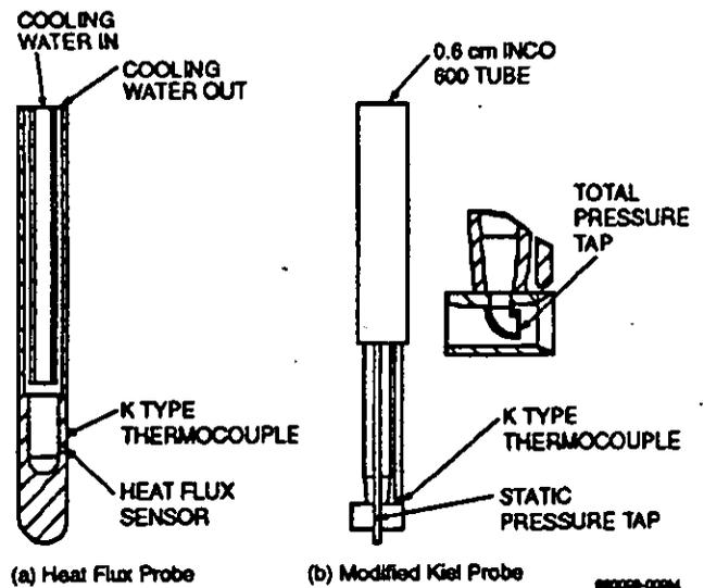
FIG. 10 - SCHEMATIC OF (a) HEAT FLUX PROBE AND (b) MODIFIED KIEL PROBE
