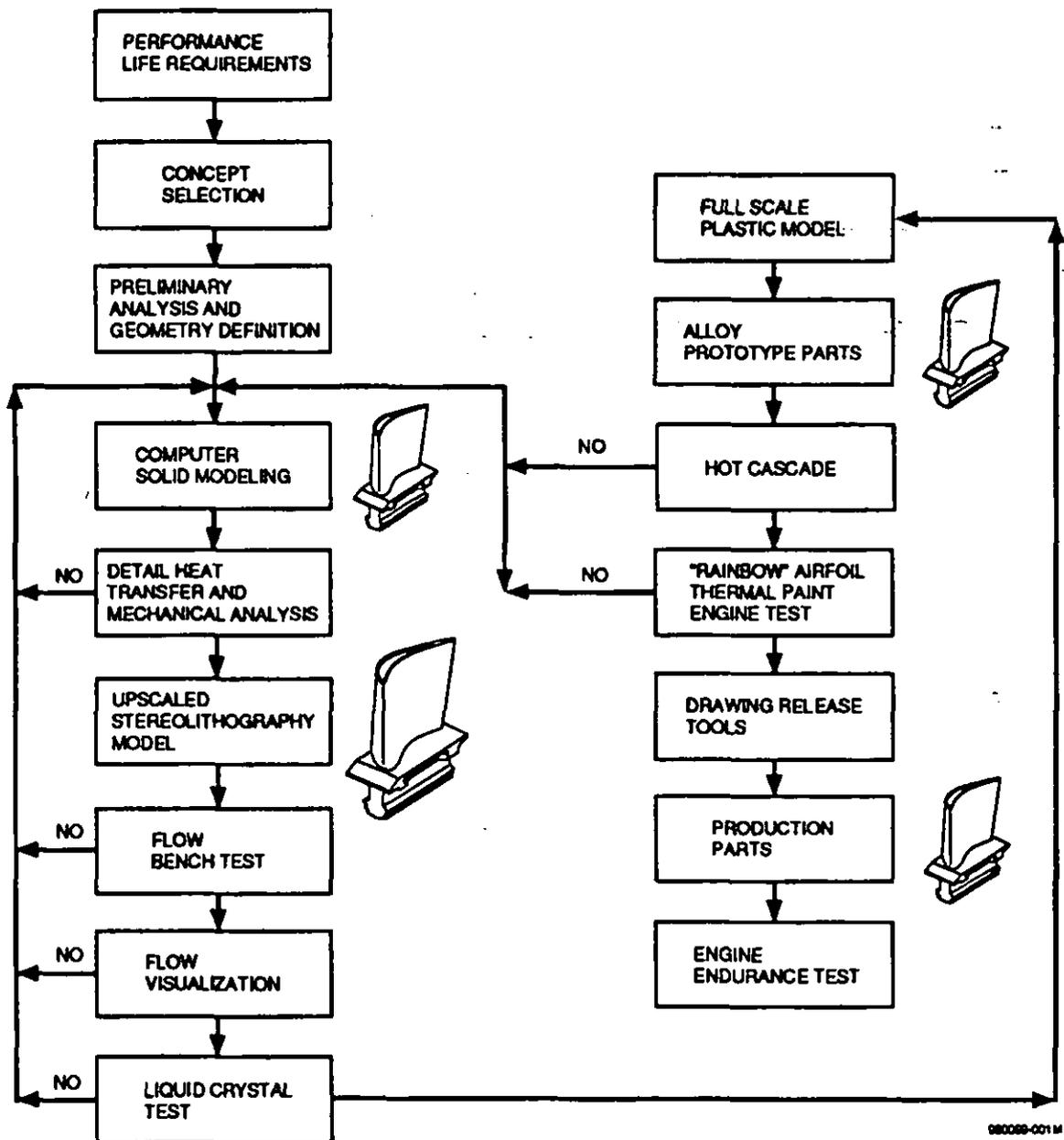
FIG. 1 - AIRFOIL COOLING DEVELOPMENT PROCESS
