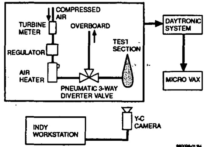
FIG. 6 - SCHEMATIC VIEW OF IMAGING TEST APPARATUS
