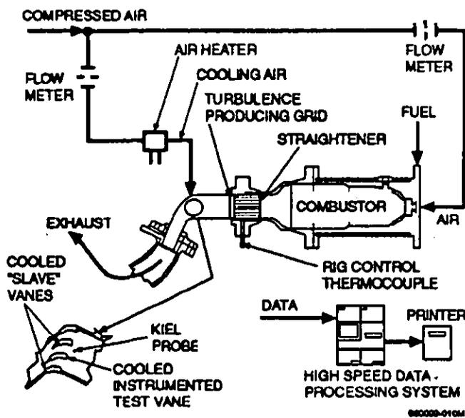
FIG. 9 - HOT CASCADE TEST RIG
