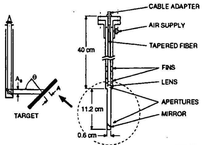
FIG. 11 - CUT-AWAY VIEW OF THE PYROMETER
