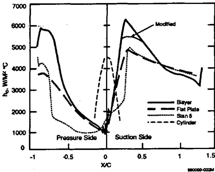
FIG. 2 - EXTERNAL HEAT TRANSFER COEFFICIENT DISTRIBUTION
