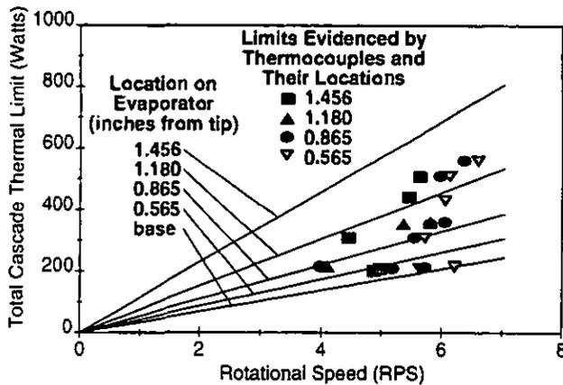
Fig. 9: Heat flux limit for TS1 with water as working fluid, as a function of rotative speed. Model results assume liquid flow rate through the inner end of the flow control insert as the limiting factor in heat flux.
