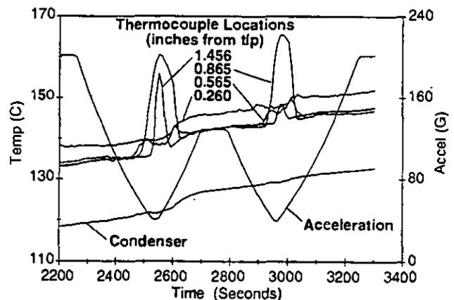
Fig. 7: Time history of an experiment with TS1 using water as a working fluid and exhibiting heat flux limit.
