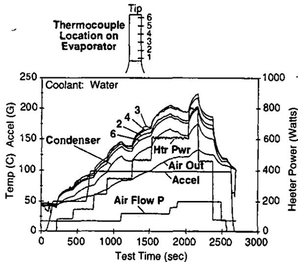
Fig. 5: Time history of an experiment with TS2 using water as working fluid.
