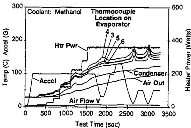
Fig. 6: Time history of an experiment with TS2 using Methanol as a working fluid and exhibiting heat flux limit.
