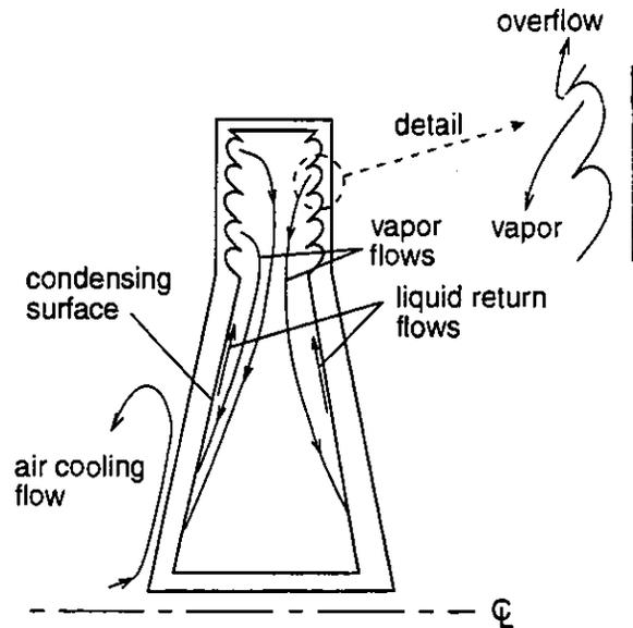
Fig. 2: Schematic diagram of evaporative-cooling system for rotor.
