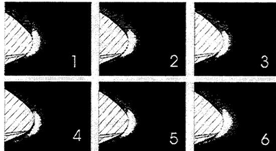
Fig. 15: Schlieren visualisation according to Fig.14 showing only little influence of pressure waves on cooling jet ( $p_{cw}/p_g = 2$ ,  $p_{pw}=3.35$  bar)
