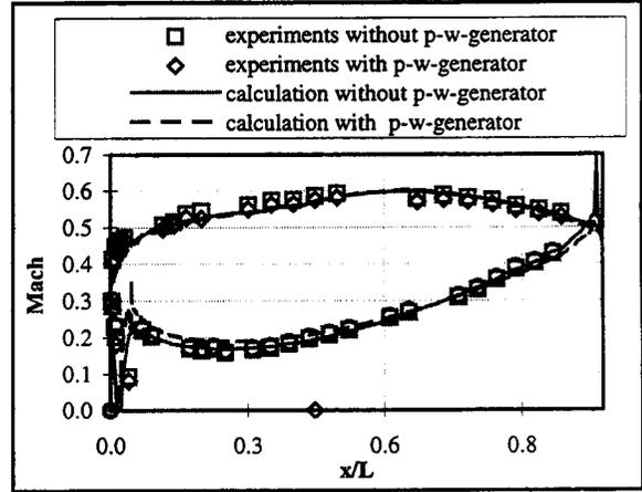
Fig. 11: Mach distribution of blade , calculation, measurements
