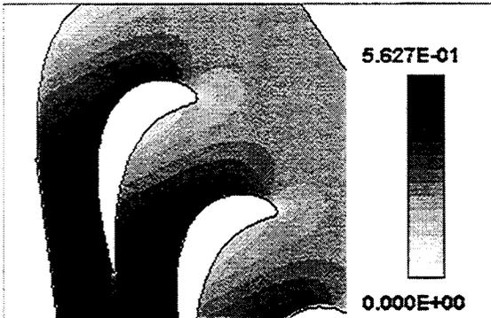
Fig. 9: Calculated test section, no pulsator, mach levels
