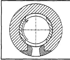
Fig. 5: Schematic drawing of the pressure wave generator
