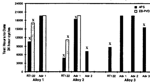
Figure 13. Advanced TBC Systems Test Results
