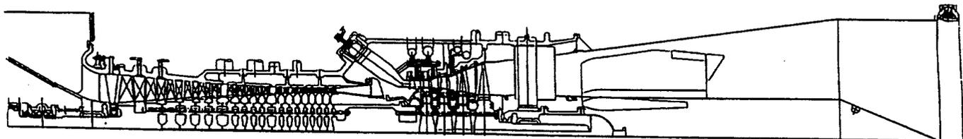
Figure 3. 501ATS Engine Cross-Section
