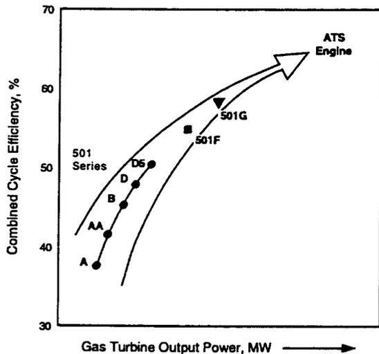
Figure 1. Evolution of Large Westinghouse Gas Turbines
