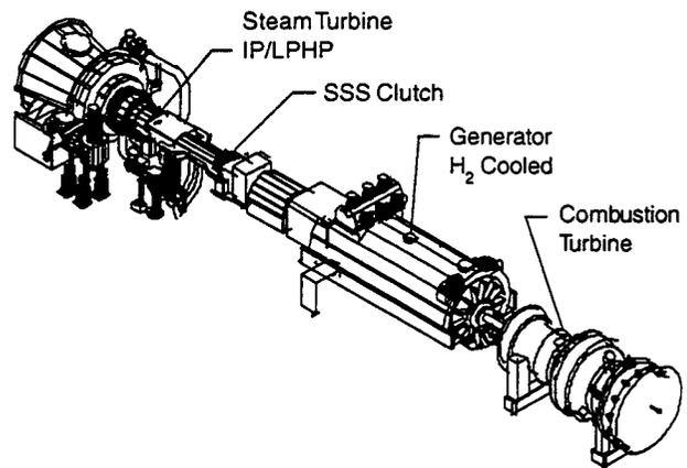
Figure 2. ATS Single Shaft Power Train
