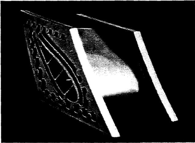
Figure 7. First Stage Vane
