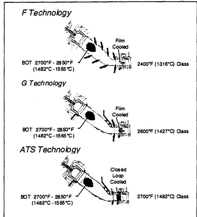
Figure 5. Closed Loop Cooling Technology
