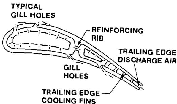
**VANE TYPE:** 2 CAVITY WITH CAST-IN TRAILING EDGE SLOTS, PIN FINs WITH EDM MACHINED GILL HOLES
