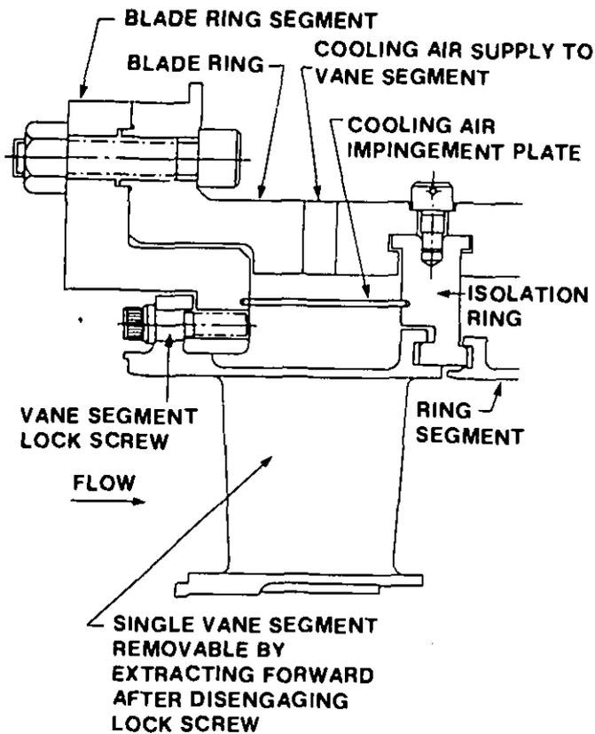
Fig. 1 Single Vane Segment
