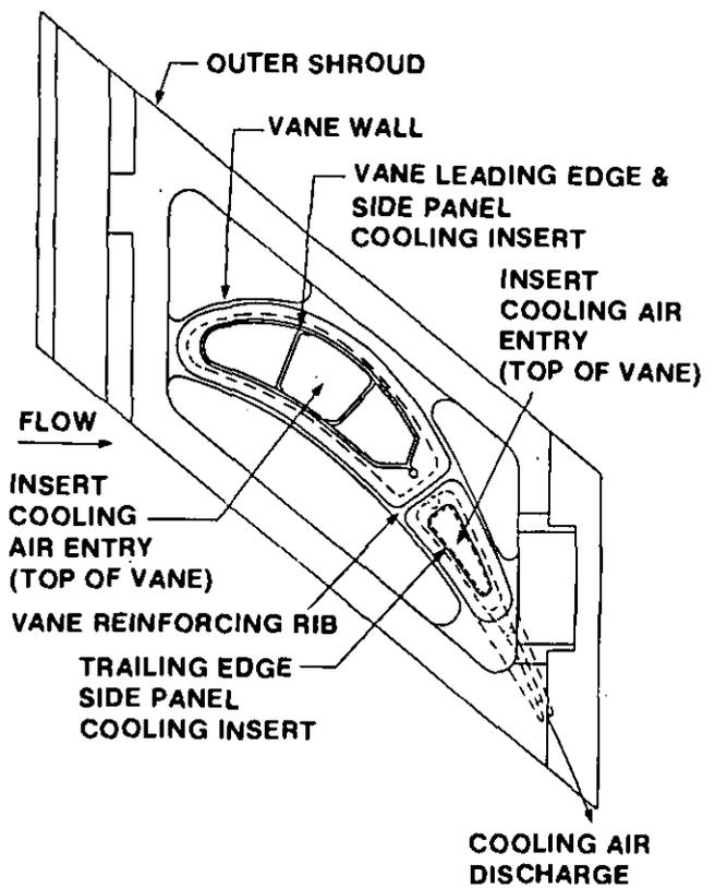
Fig. 2 Top View of Vane Showing Inserts
