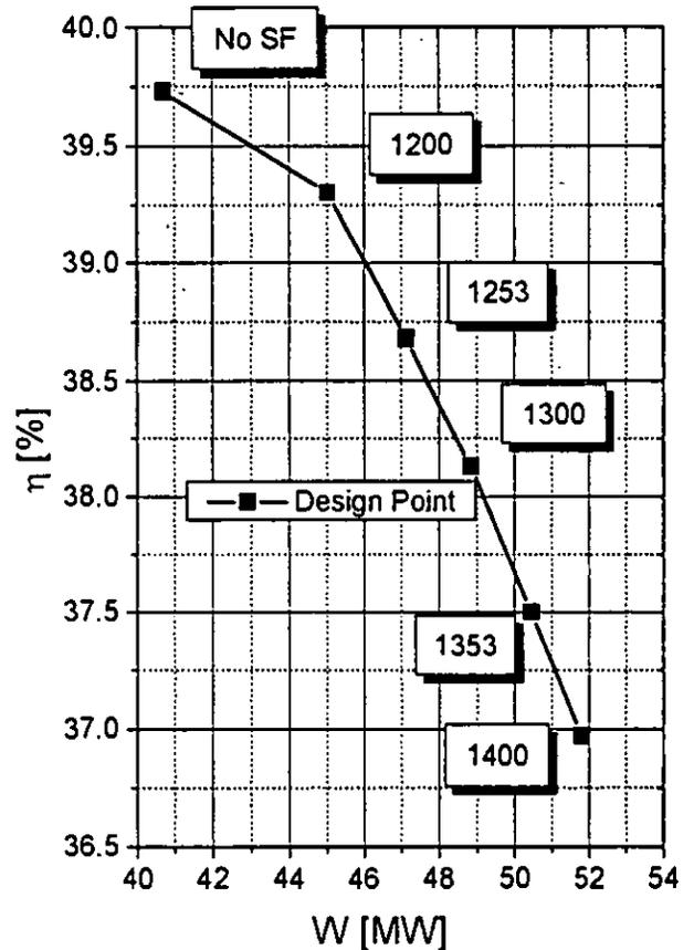
Figure 8: Efficiency/Power Trend at Various Supplementary Fairing Temperature for the LM6000-SF
