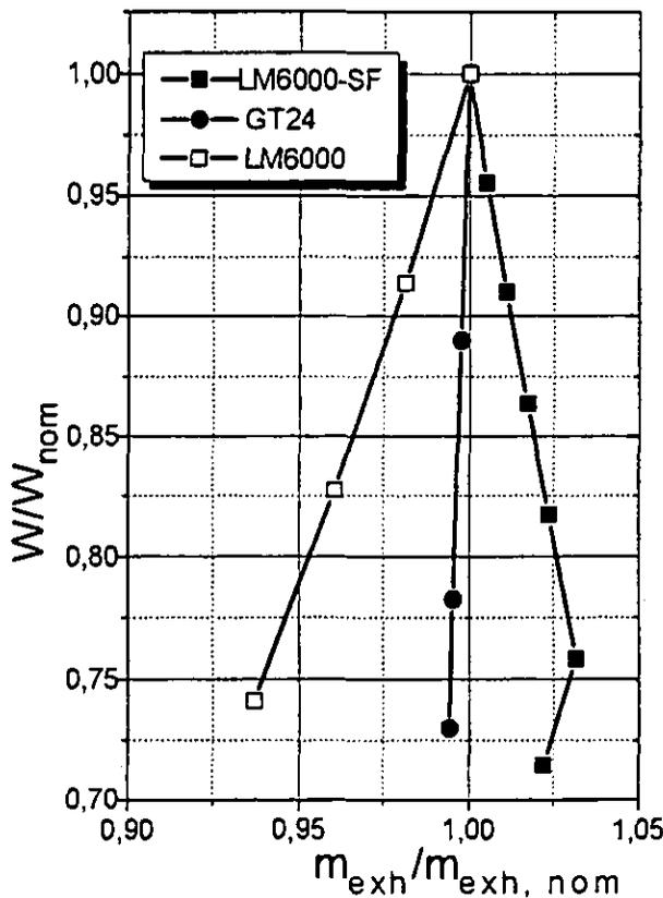
Figure 13: Power Vs. Exhaust Gas Mass Flowrate. LM6000, GT24 and LM6000-SF Comparison
