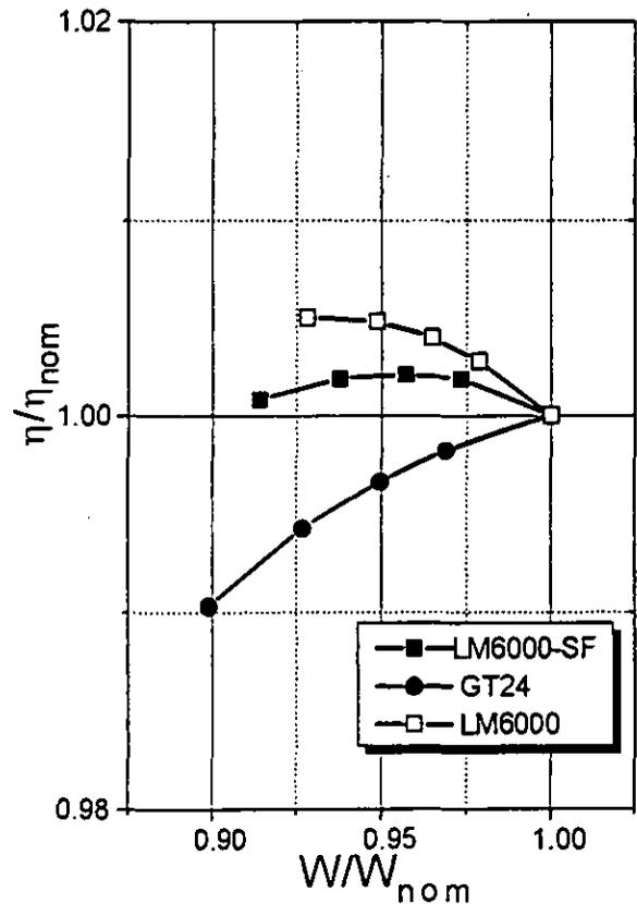
Figure 14: Efficiency/Power Trend with IGVC. LM6000, GT24 and LM6000-SF Comparison
