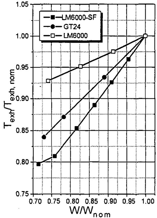
Figure 12: Exhaust Gas Temperature Vs. Power. LM6000, GT24 and LM6000-SF Comparison
