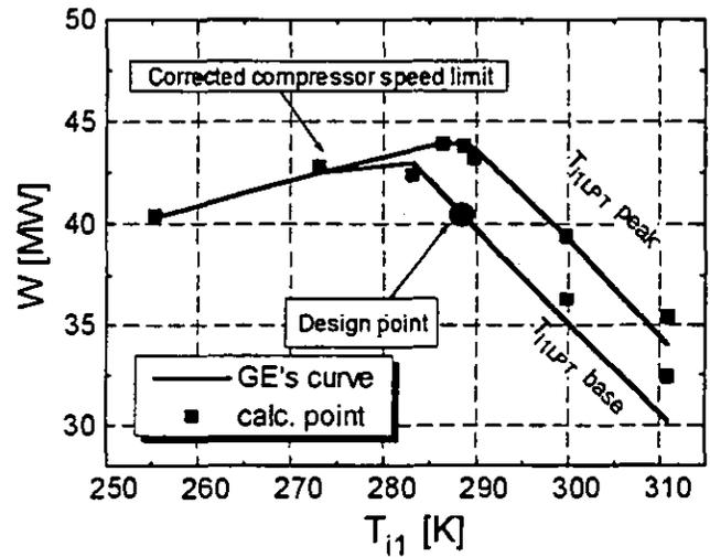
Figure 5: Power Output Vs. Compressor Inlet Temperature. Calculated Data and Constructor Curves Comparison
