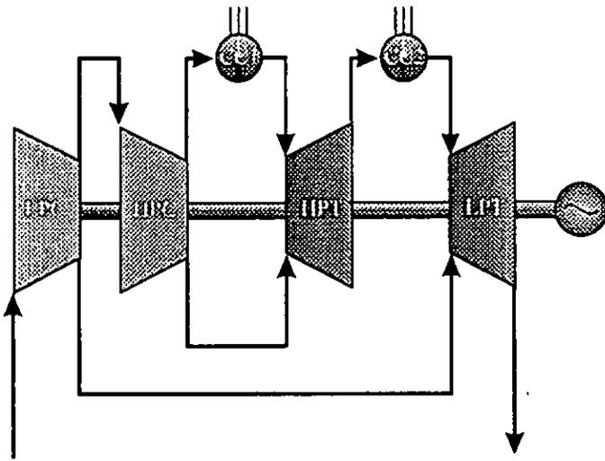
Figure 6: Simulation Model of GT24 Gas Turbine
