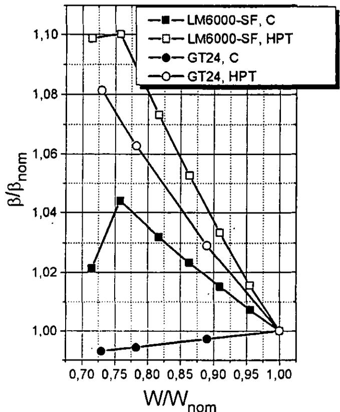
Figure 10: Compression and Expansion Ratio Vs. Power.
