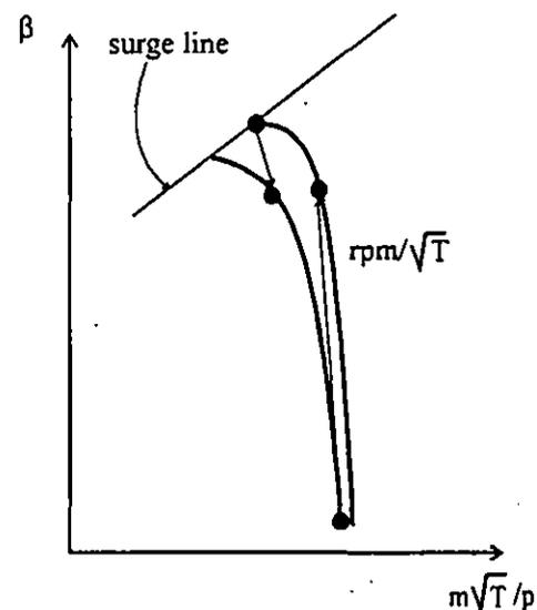
Figure 3: Axial Compressor Characteristic Curves: Instability Control
