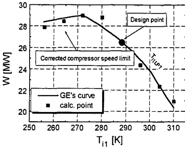
Figure 4: Power Output Vs. Inlet Compressor Temperature. Results and Constructor Curves Comparison.
