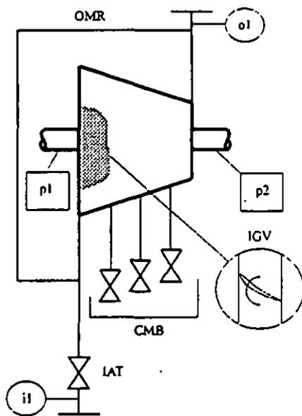
Figure 2: Axial Compressor Module With Control Systems.
