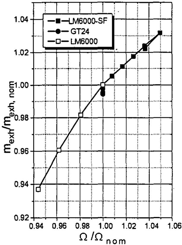
Figure 11: Exhaust Gas Mass Flowrate Vs. Shaft Speed. LM6000, GT24 and LM6000-SF Comparison
