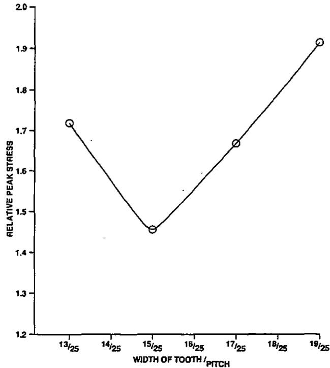
FIG. 17. STRESS VERSUS WIDTH OF TOOTH/PITCH
