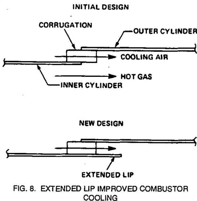
FIG. 8. EXTENDED LIP IMPROVED COMBUSTOR COOLING
