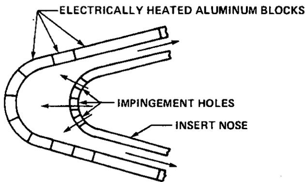
FIG. 14. INSERT NOSE IN THE LEADING EDGE HEAT TRANSFER RIG
