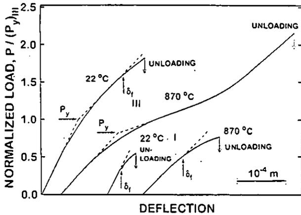
Figure 7. Load vs. deflection curves observed in coated SP specimens (zones I and III) tested at 22 °C and 870 °C indicating yield load ( $P_y$ ) and critical deflection to cracking ( $\delta_f$ ). The load is normalized by yield load of region III at RT.
