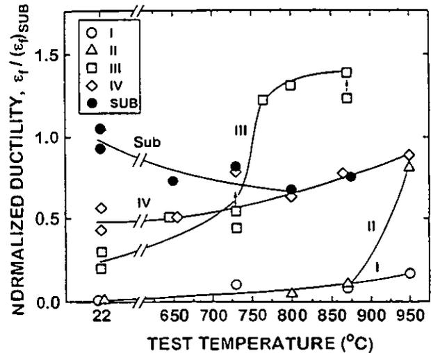
Figure 10. Temperature dependence of ductility ( $\epsilon_f$ ) in coating regions I-IV and substrate. The ductility is normalized by that in substrate at RT.
