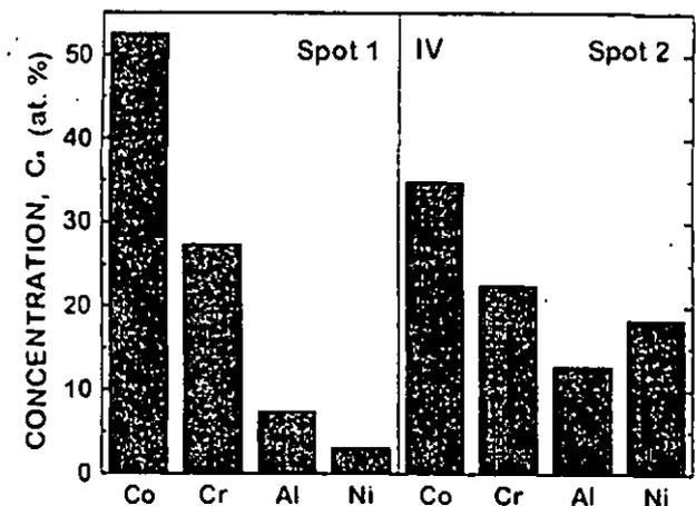
Figure 6. Chemical composition of coating region IV adjacent to region III (spot 1) and substrate (spot 2).
