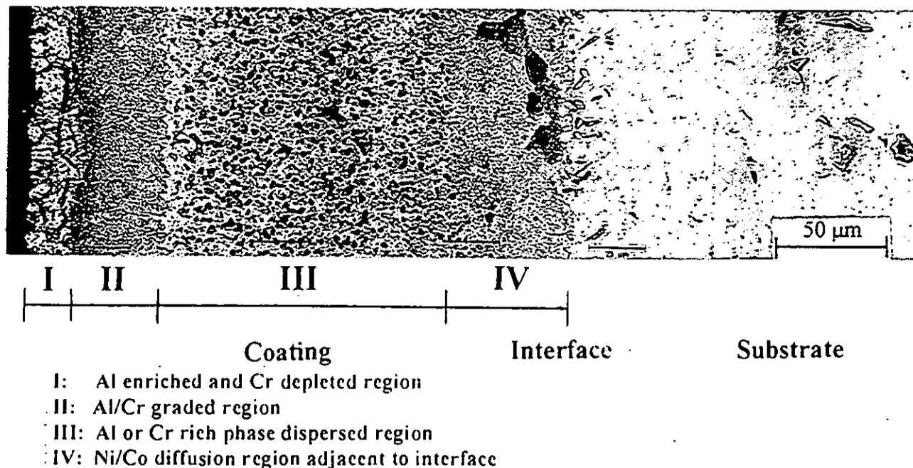
Figure 1. Micrograph indicating layered structure of aluminized coating divided into four regions (I-IV).
