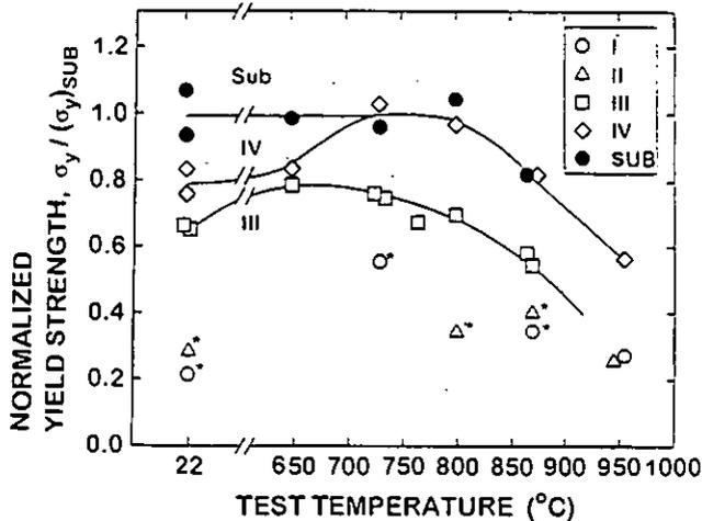
Figure 8. Temperature dependence of yield strength ( $\sigma_y$ ) in coating zones III and IV and substrate. An asterisk mark indicates the fracture strength for coating regions I and II. The yield and fracture strength are normalized by  $\sigma_y$  in substrate at RT.
