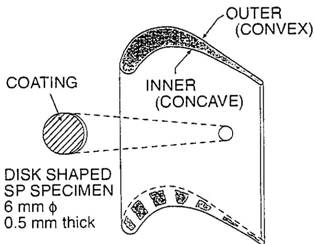
Figure 2. Extraction of disk-shaped small punch (SP) specimens from gas turbine blades.
