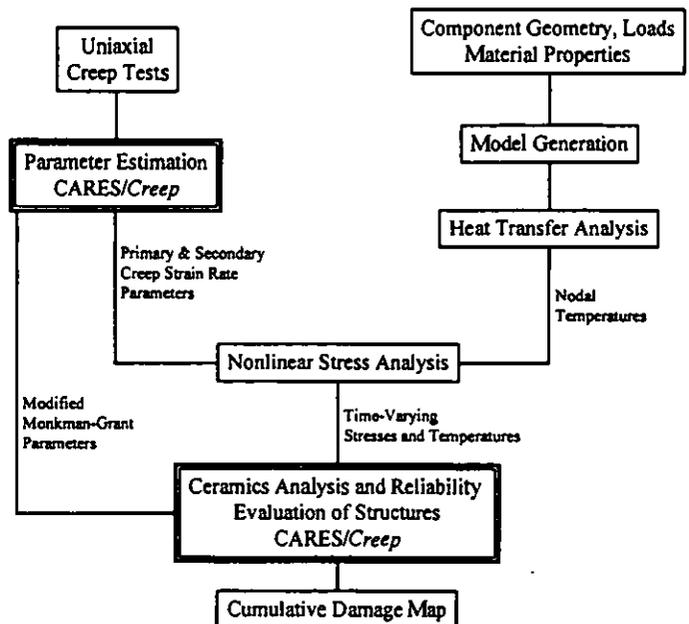
Figure 1 Block diagram for the analysis of a monolithic ceramic components using CARES/Creep.
