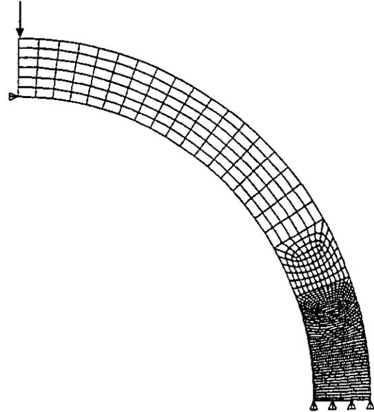
Figure 6 Finite element mesh for the C-ring.
