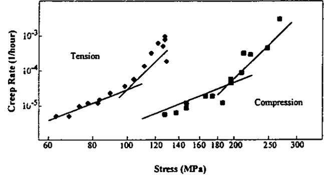
Figure 2 Creep rate vs. stress for the siliconized silicon carbide material tested in tension and compression (Wiederhorn, et al., 1988).
