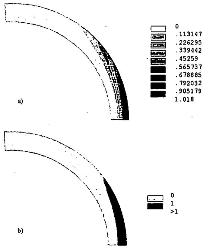
Figure 8 Cumulative damage in the C-ring at a) time equal to  $t_1$  and b) time equal to  $t_2$ .
