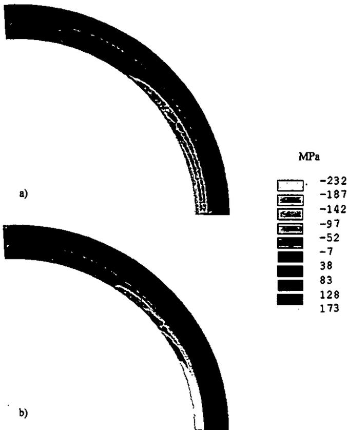
Figure 7 Tangential stress distribution in the C-ring at time equal to a) zero and b)  $t_1$  hours, where the maximum tensile stress is 172 and 96 MPa, respectively.
