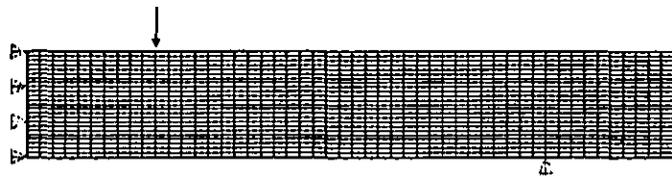
Figure 3 Finite element mesh for the 4-pt bend specimen.
