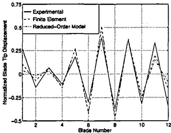
**Fig. 15** Comparison of experimental, finite element, and ROM mistuned mode shapes at 256 Hz.
