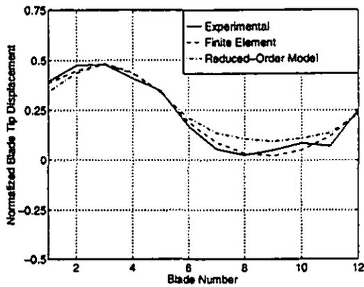
**Fig. 13** Comparison of experimental, finite element, and ROM mistuned mode shapes at 311 Hz. Note that out-of-plane blade modes, which reside in moderate modal density areas, are more sensitive to mistuning than disk-dominated modes.
