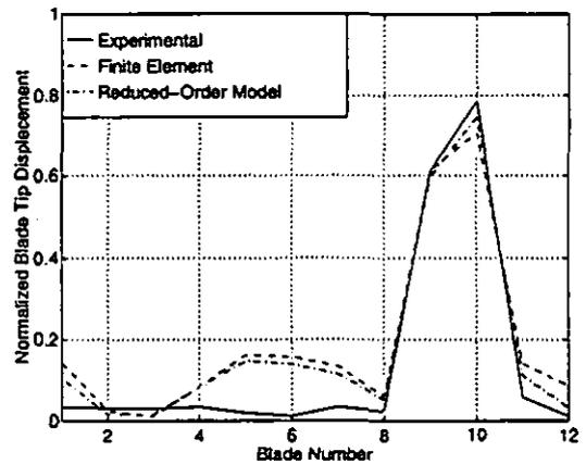
**Fig. 18** Comparison of experimental, finite element, and ROM mistuned modes at 908 Hz.
