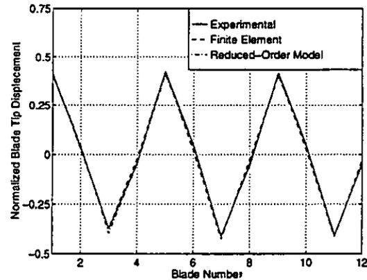
**Fig. 12 Comparison of experimental, finite element, and ROM mistuned modes shapes at 523 Hz. Note that disk-dominated modes, which reside in low modal density areas, are largely insensitive to mistuning effects.**
