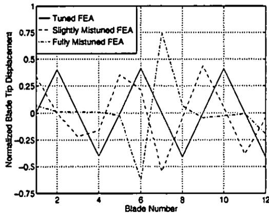
**Fig. 10** Effect of blade length mistuning, as predicted by finite element analysis (FEA), on the three nodal diameter in-plane blade mode at 917 Hz.
