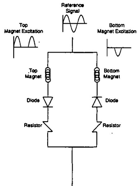
Fig. 3 Diode circuit used to block negative and positive current flows into the top and bottom magnets, respectively.
