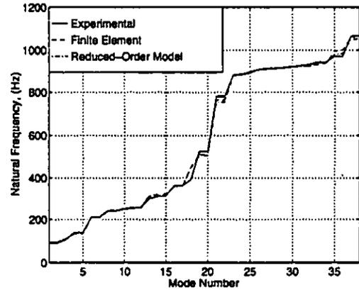
**Fig. 11** Natural frequencies for the mistuned bladed disk versus the mode number. Note that the nodal description is no longer a valid manner in which to describe the mistuned mode shapes.
