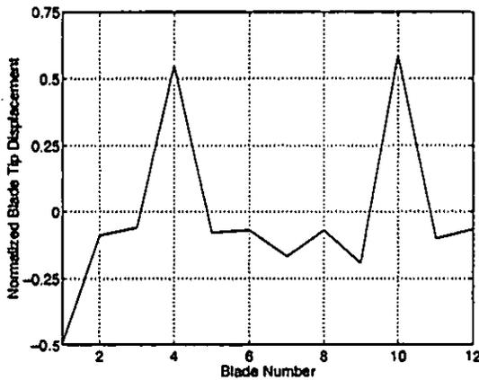
**Fig. 9** In-plane blade mode, measured experimentally at 917 Hz for the nominally tuned bladed disk.
