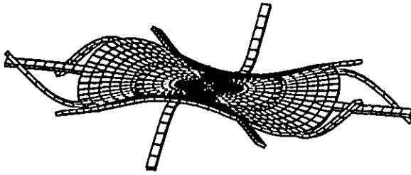
Fig. 5 Tuned three nodal diameter mode at 514 Hz. Disk-induced and cantilever blade motion dominate this mode shape.
