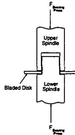
Fig. 2 Section view of the bladed disk-spindle connection.
