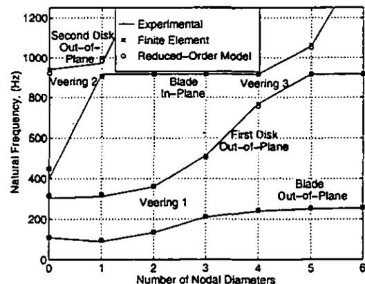
**Fig. 4 Tuned natural frequencies versus number of nodal diameters. Note the excellent agreement between experimental, finite element, and ROM natural frequencies.**
