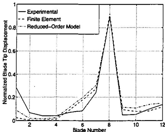
Fig. 21 Comparison of experimental, finite element, and ROM mistuned modes at 932 Hz.
