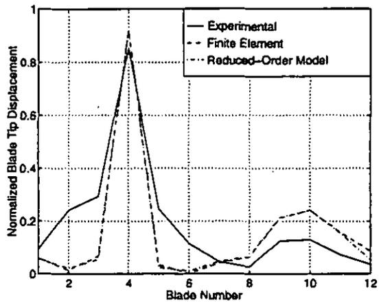
**Fig. 17** Comparison of experimental, finite element, and ROM mistuned modes at 898 Hz.
