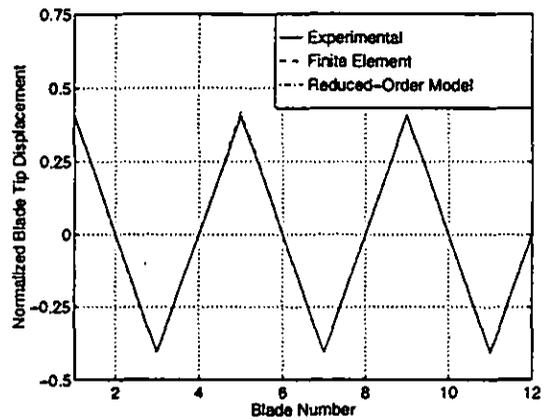
Fig. 8 Comparison of experimental, finite element, and ROM three nodal diameter tuned mode shapes at 210 Hz.
