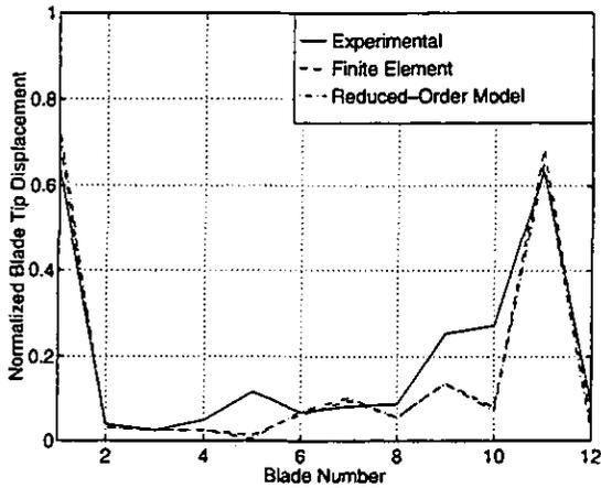
Fig. 19 Comparison of experimental, finite element, and ROM mistuned modes at 918 Hz.
