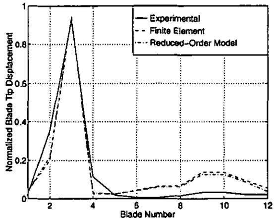
**Fig. 16** Comparison of experimental, finite element, and ROM mistuned modes at 882 Hz.
