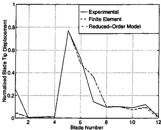
Fig. 20 Comparison of experimental, finite element, and ROM mistuned modes at 921 Hz.
