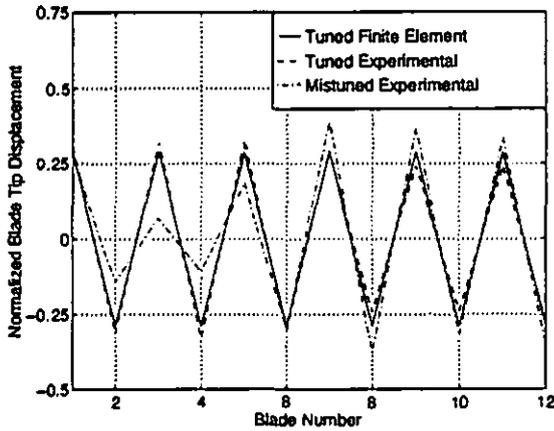
**Fig. 14** Comparison of finite element and experimental six nodal diameter tuned modes shapes at 255 Hz with the experimental six nodal diameter mode shape of the mistuned test specimen at 256 Hz.
