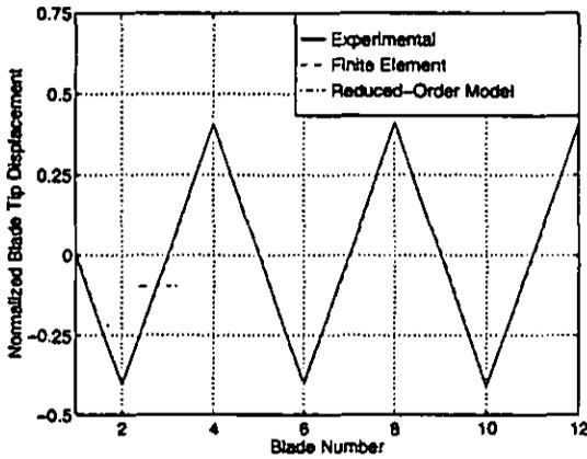
Fig. 6 Comparison of experimental, finite element, and ROM three nodal diameter tuned mode shapes at 514 Hz.
