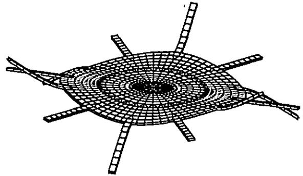
Fig. 7 Tuned three nodal diameter mode at 210 Hz. Cantilever blade motion dominates this mode shape.
