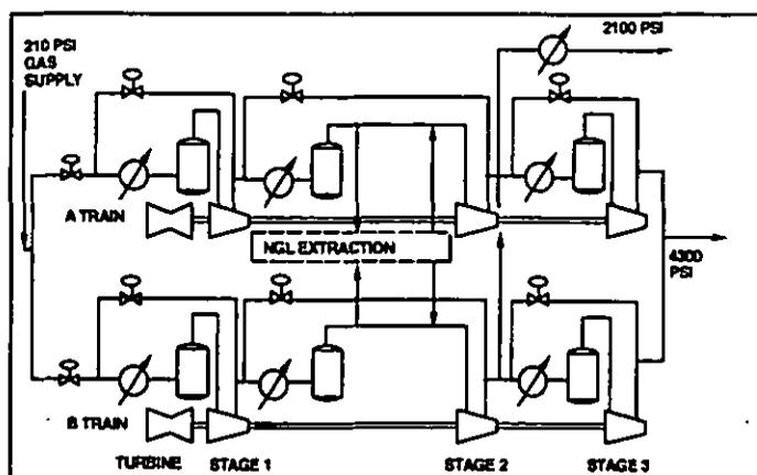
Figure 1. Three stage parallel train compression process with natural gas liquids extraction after first stage. Intermediate gas extraction after second and third stage.
