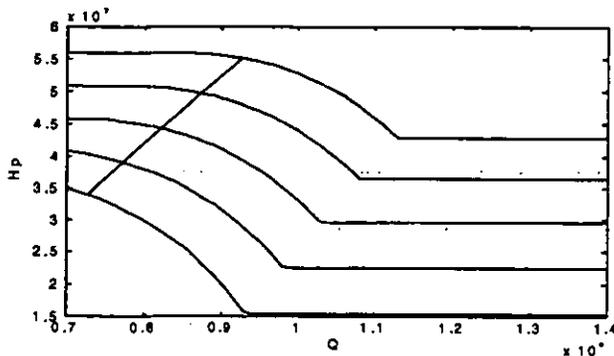
Figure 2. Polytropic Head (ft.lbf/lbm) vs. Flow (ACFM) for speeds 0.85, 0.90, 0.95, 1.0, 1.05
