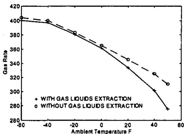
Figure 5. Third Stage Gas Rate ( $10^6$  SCFD) versus Ambient Temperature ( $^{\circ}$ F)
