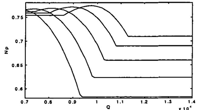
Figure 3. Polytropic Efficiency vs. Flow (ACFM) for speeds 0.85, 0.90, 0.95, 1.0, 1.05
