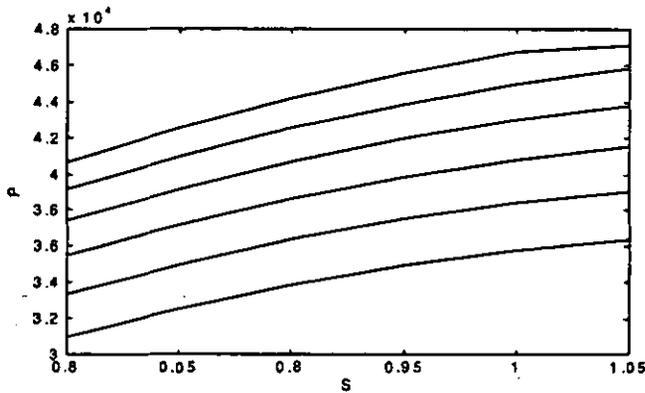
Figure 4. Maximum Turbine Power (HP) vs. Speed (1=100%) for Ambient Temperatures (-40, -20, 0, 20, 40, 60 °F)
