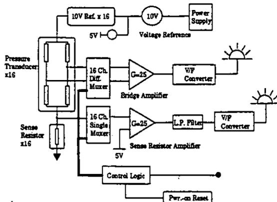
Fig. 7: DLR Pressure transducer circuit block diagram
