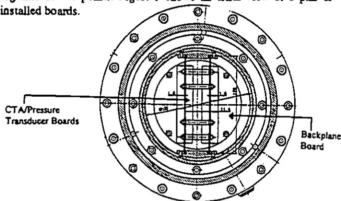
Fig. 9: End View of Backplane board in the DLR turbine shaft. (Drawing courtesy DLR)
