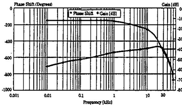
Fig. 5: CTB circuit gain and phase response curves showing a bandwidth of 30 kHz at the 3 dB point.
