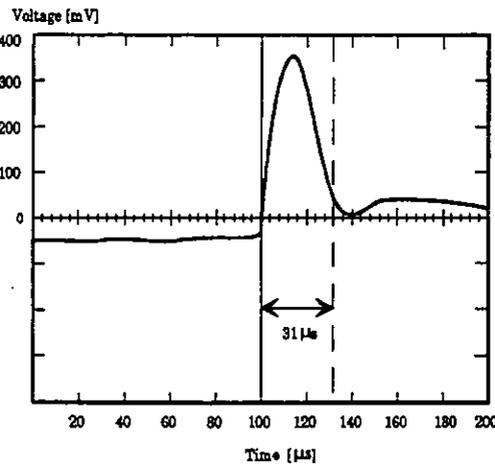
Fig. 6: CTB Square wave response curve showing approximately a 30 kHz bandwidth
