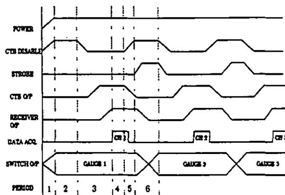
Fig. 4: CTB timing diagram showing the phase relationship between channel data acquisition and gauge switching.
