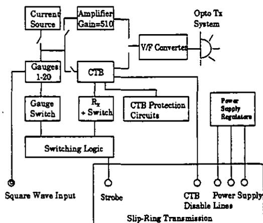
Fig. 3: CTB block diagram.
