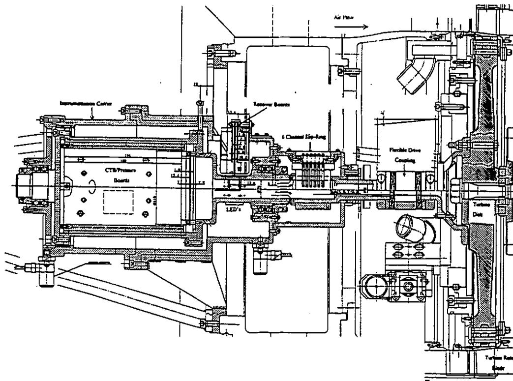
Fig. 1: Core of DLR turbine facility
