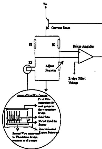
Fig. 2: Basic CTB block diagram.
