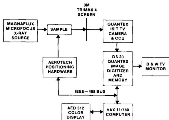
Fig. 1 Block diagram of the tomographic system.
