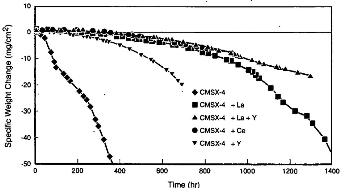
Figure 10 - 1093°C (2000°F) dynamic oxidation test results for Bare CMSX-4 with RE additions and without.
