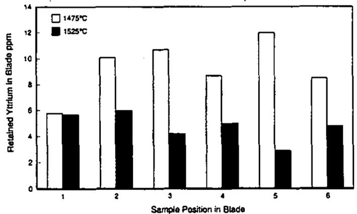
Figure 4 - Retained yttrium in cored blades.
