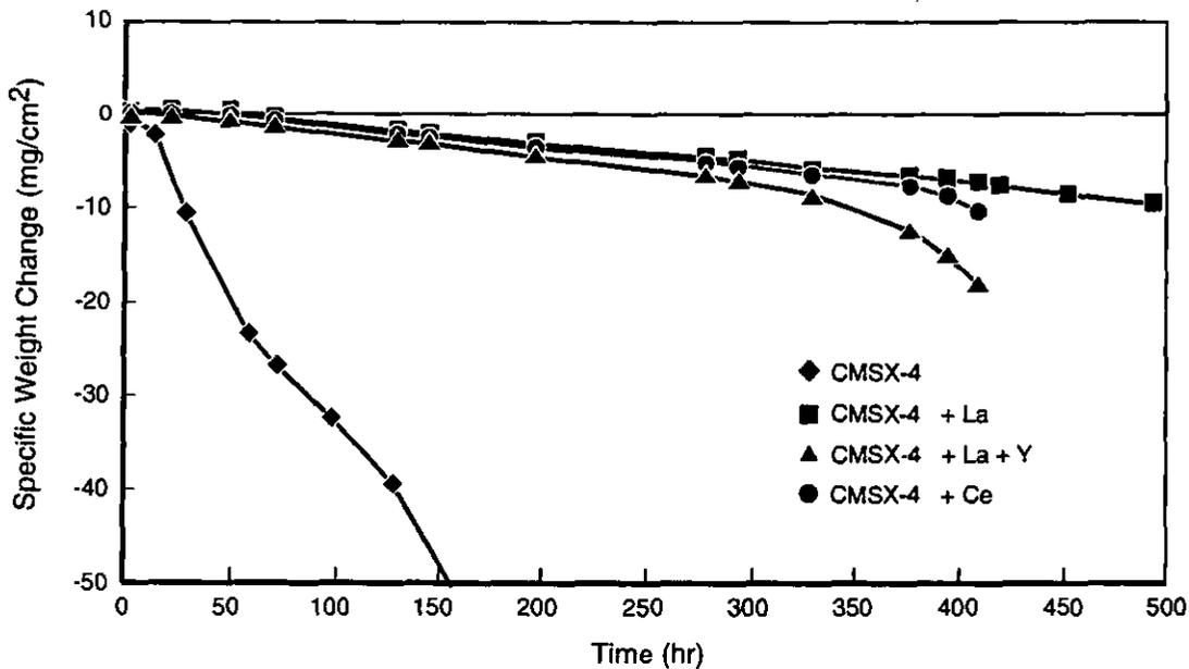
**Figure 11 - 1149°C (2100°F) dynamic oxidation test results for Bare CMSX-4 with RE additions and without.**
