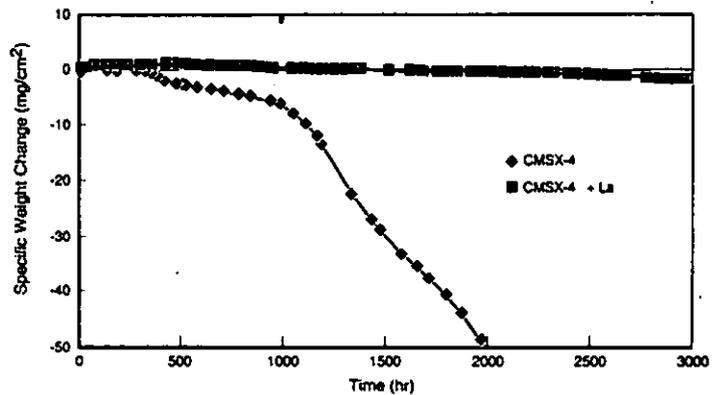
Figure 9 - 1038°C (1900°F) dynamic oxidation test results for Bare CMSX-4 with La addition and without.
