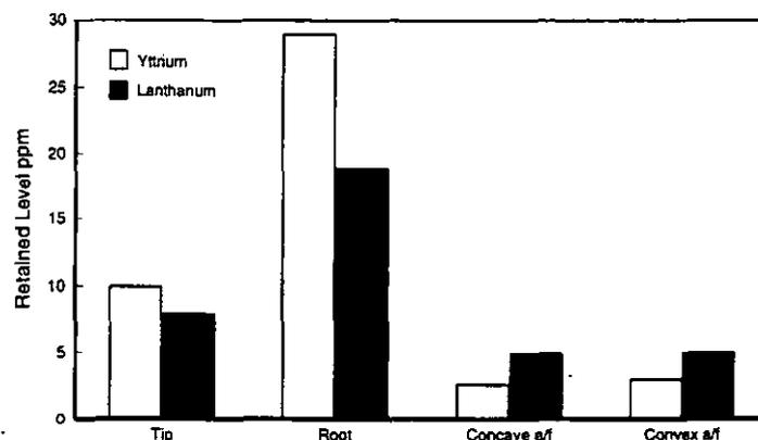
Figure 8 - Retained yttrium and lanthanum in turbine blades.
