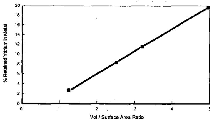
Figure 5 - Effect of surface area on level of retained yttrium.
