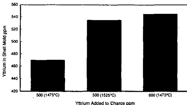
Figure 6 - Yttrium in shell molds cast at different temperatures.
