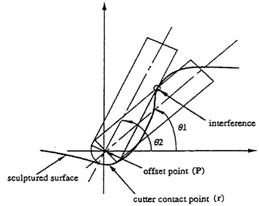
Fig. 4 Schematic illustration of rotational range of a cutter and interference
