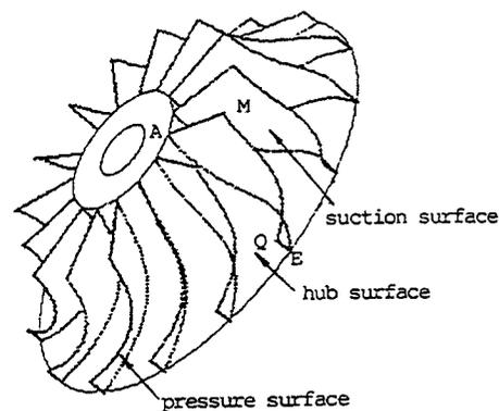
**Fig. 7 Schematic illustration of a fifteen-blade impeller**
