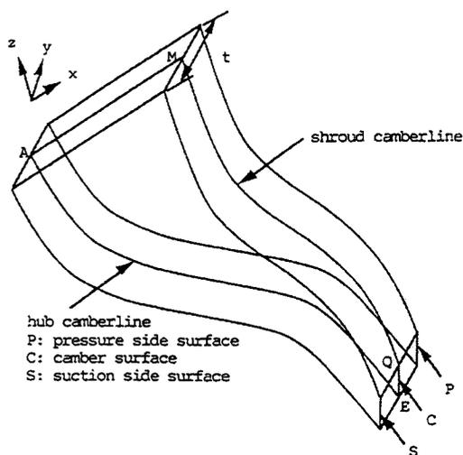
**Fig. 6 Schematic illustration of camber, pressure side, and suction side surfaces of an impeller**
