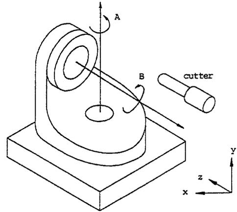
Fig. 5 Schematic illustration of a different type of five-axis machining
