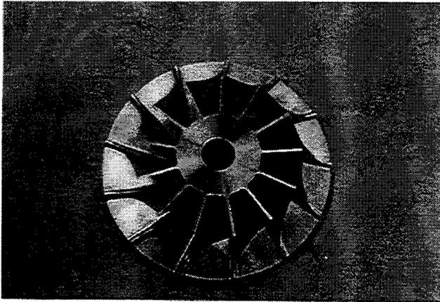
**Fig. 12 A machined impeller with thirteen blades**
