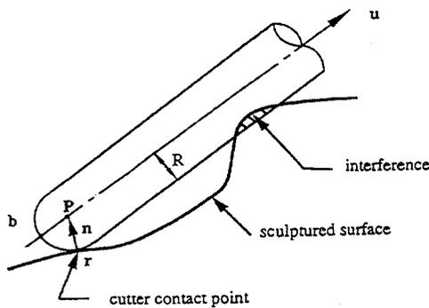
Fig. 2 Schematic illustration of interference and cutter location
