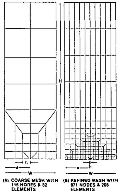
Fig. 1. 2-D Mesh Idealizations used for Modeling the Single Edge Crack (Sec) Specimen.
