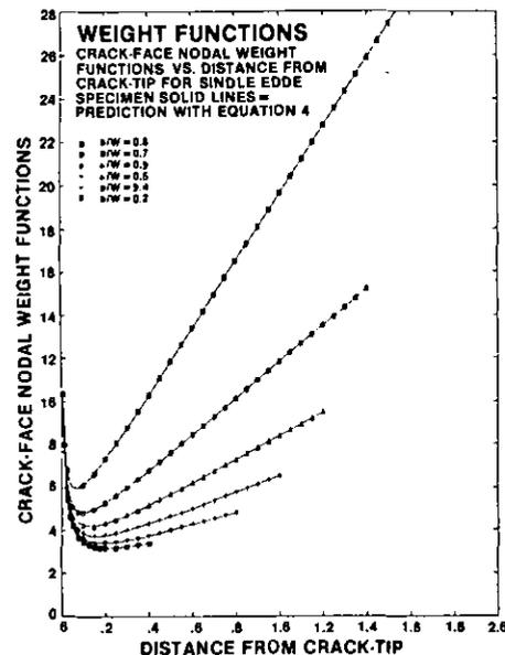
Fig. 8. Comparison between Fitted and Calculated Crack-Face Nodal Weight Functions as a Function of Crack-Face Distance for Sec Specimen with different  $\frac{a}{W}$  ratios.
