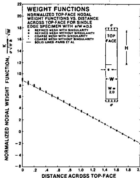
Fig. 4. Normalized Nodal Weight Functions Across the Top-Face for Single Edge Crack Geometry with  $\frac{a}{w} = 0.5$ .
