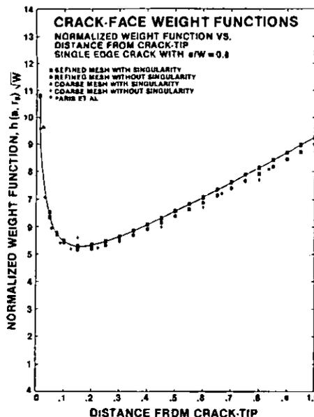
Fig. 5. Normalized Crack-Face Nodal Weight Functions as a Function of Distance from Crack-Tip with and without Singular Elements for Sec Specimen with  $\frac{a}{w} = 0.5$ .
