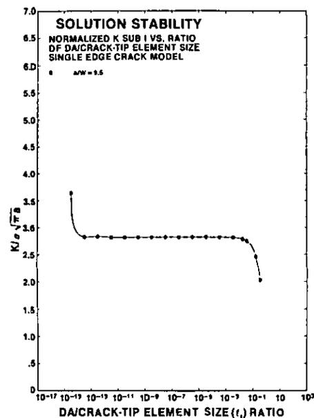
Fig. 2. Effect of Incremental Crack Size ( $\Delta a$ ) of Virtual Crack Extension on Solution Stability;  $K_I / \sigma \sqrt{\pi a}$  vs.  $\Delta a / k_s$  ratios.
