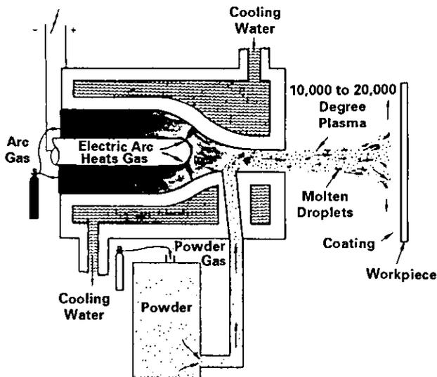
Fig. 2 Plasma Deposited TBC Process Schematic.
