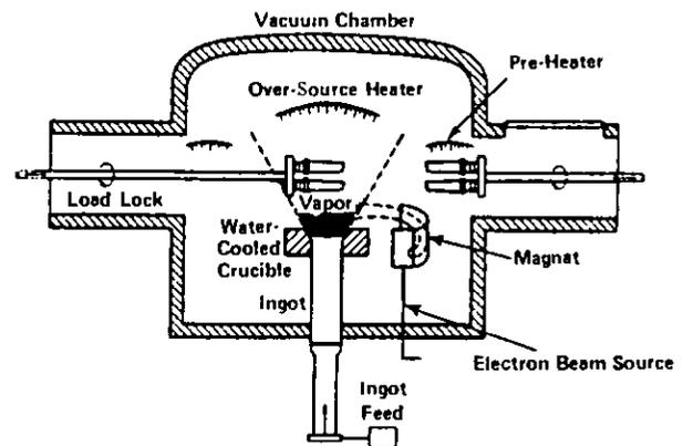
Fig. 4 Electron Beam-Physical Vapor Deposited TBC Process Schematic.
