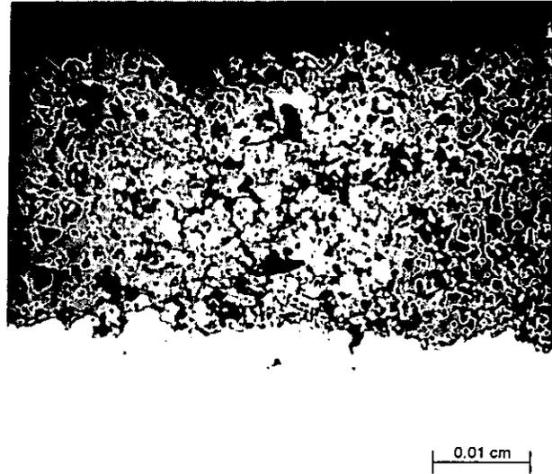
Fig. 3 The Microstructure of Air Plasma Deposited 7 Weight Percent Ytria Partially Stabilized Zirconia.
