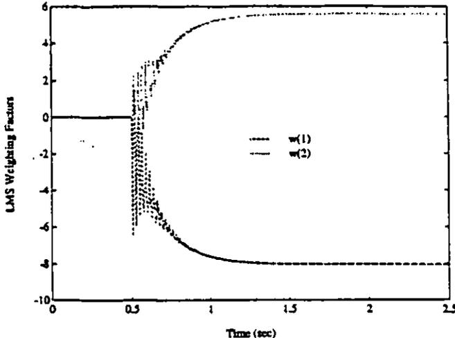
Figure 14. FIR filter coefficients (65 Hz case).
