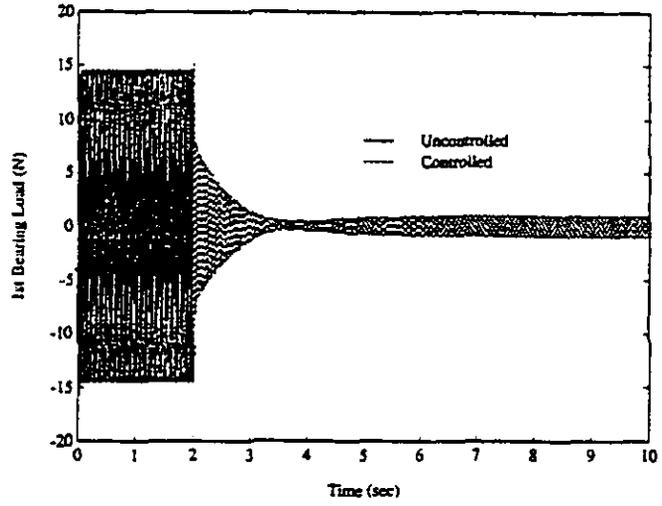
Figure 9. 1st Bearing load from FEM (30 Hz case).
