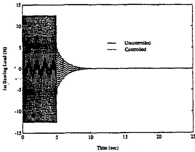
Figure 7. 1st Bearing load from DCM (10 Hz case).
