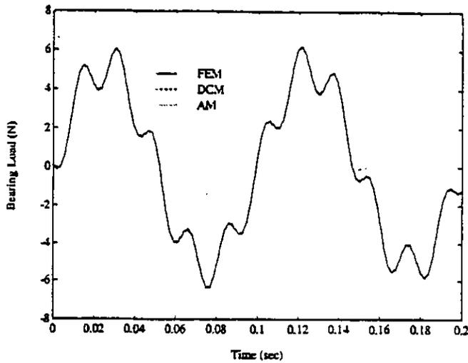
Figure 2. Reaction force in simply-supported beam.
