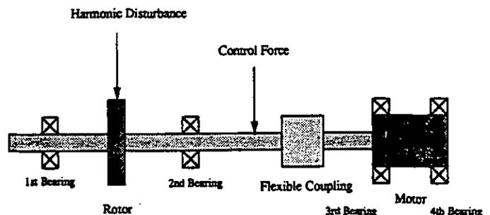
Figure 5. Illustration of rotating machinery system.
