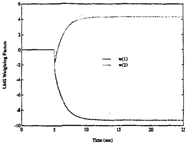
Figure 8. FIR filter coefficients (10 Hz case).
