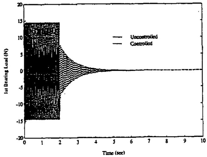
Figure 10. 1st Bearing load from DCM (30 Hz case).
