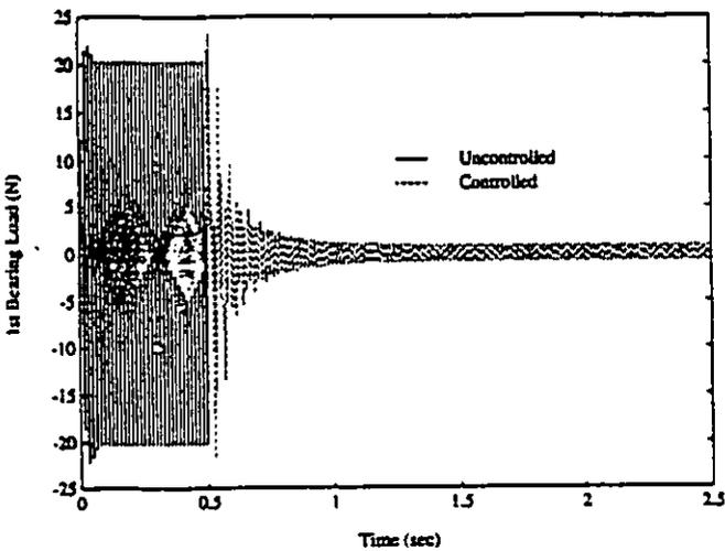
Figure 12. 1st Bearing load from FEM (65 Hz case).
