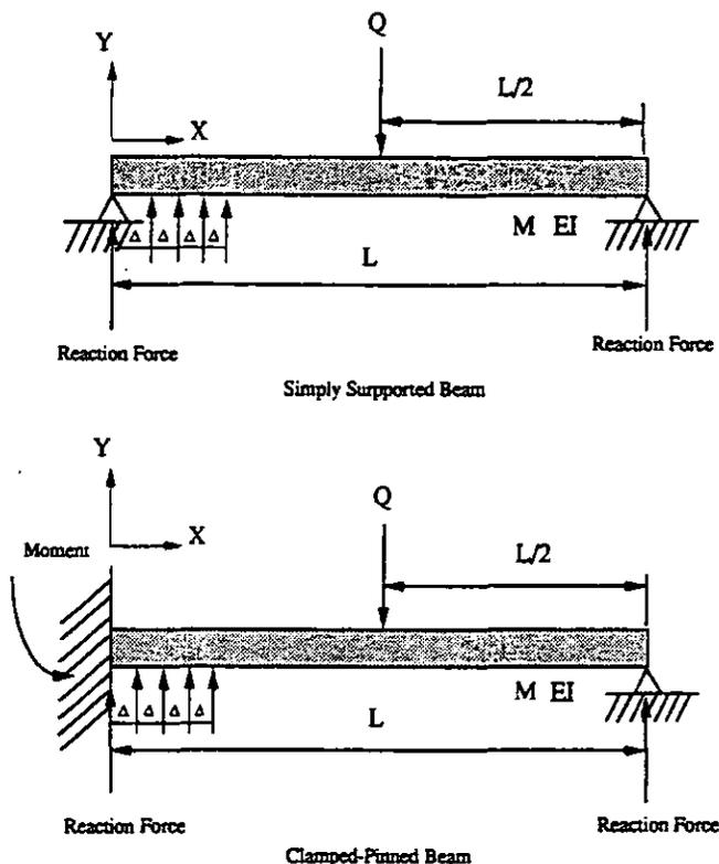
Figure 1. Simply-supported and clamped-pinned beams.
