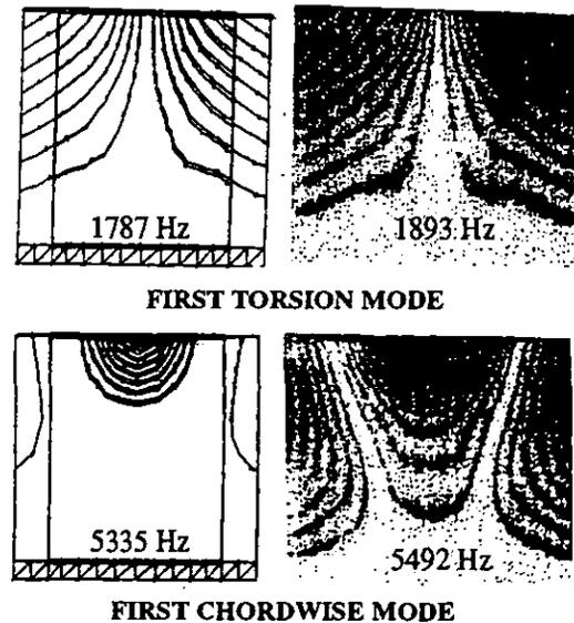
Figure 3: Comparison Between NASTRAN and Holographic Mode Shapes for Specimen PW12
