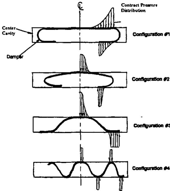
Figure 4: Damper Configurations
