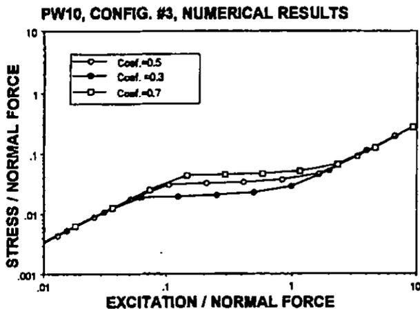
Figure 11: Predicted Damper Performance Using Micro-Slip Model
