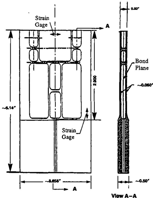
Figure 1: Hollow Specimen W/StrainGage Locations Identified
