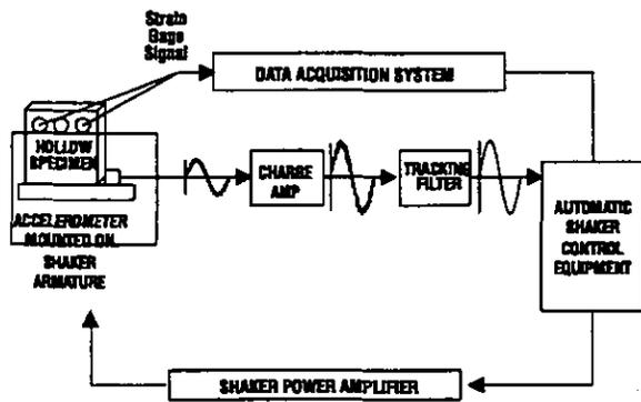
Figure 7: Block Diagram of Shaker Table Control Loop and Data Acquisition System
