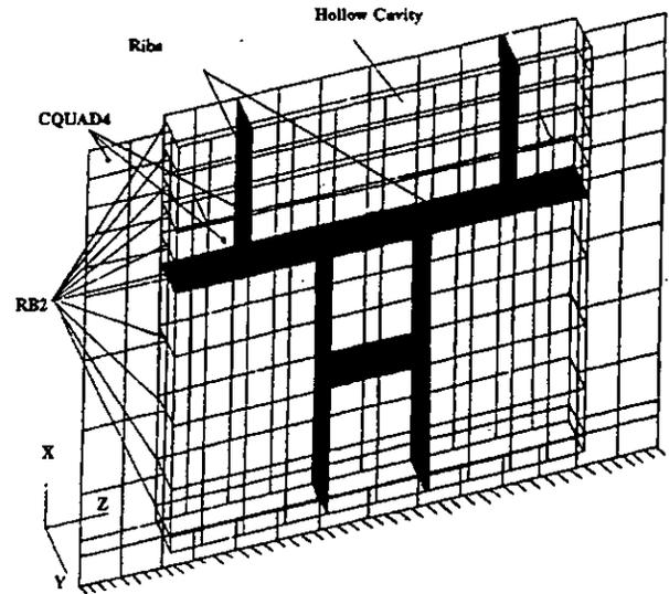
Figure 2: Finite Element Model For Hollow Specimens
