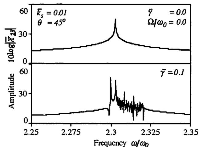
Figure 6 Variation of frequency response of systems with and without a crack
