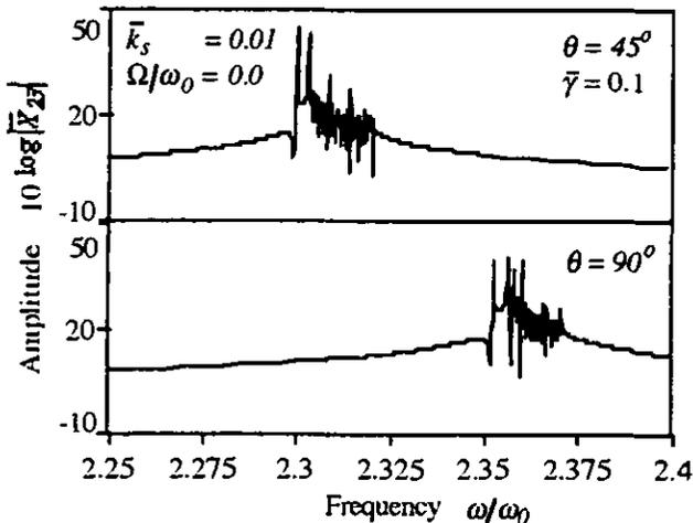
**Figure 7** Variation of frequency response of systems with and without considering the rotational speed effect
