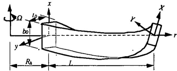
(b) Geometry of the pretwisted taper blade
