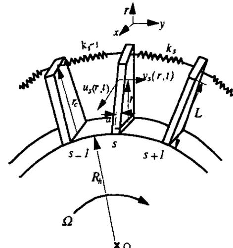
(a) Geometry of the blade-disk system
