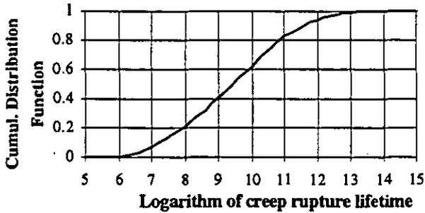
Figure 7: Distribution Function of Creep Rupture Lifetime
