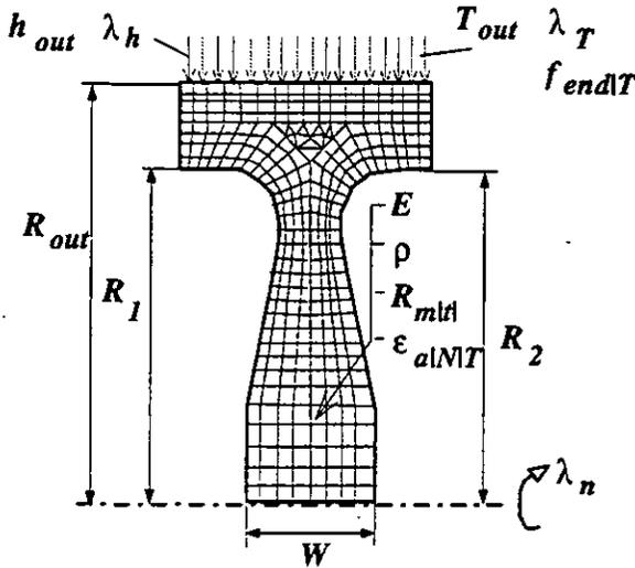
Figure 4: Sketch of FE model of turbine disk
