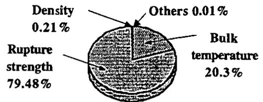
Figure 5: Probabilistic importance measures for rupture lifetime
