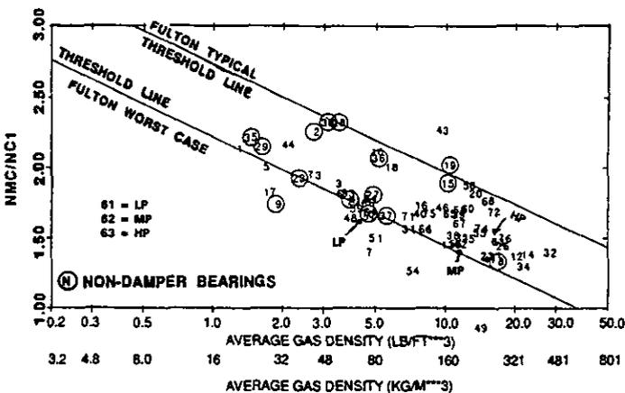
Fig. 6 - Flexibility Ratio With Tilt Pad Seals Vs. Average Gas Density
