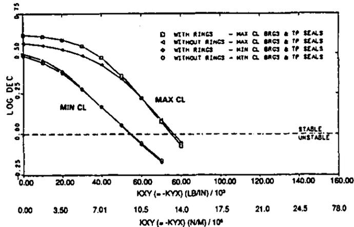
Fig. 8 - Log Dec Vs. Aero. Excitation With and Without Outer Ring Seal - No Labys
