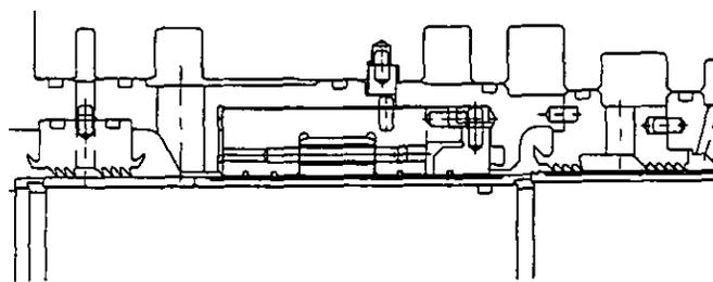
Fig. 3 - Tilt Pad Seal
