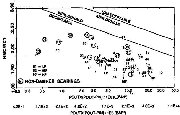
Fig. 7 - Flexibility Ratio With Tilt Pad Seals Vs. Discharge Pressure X (Discharge - inlet Pressure)
