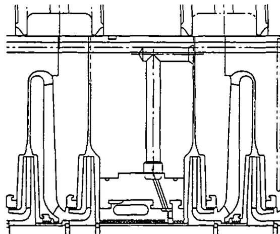
Fig. 5 - Shunt Holes & Honeycomb Seal At The Division Wall
