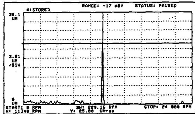
Fig. 10 - Spectrum Plot - 272B4/4 Compressor
