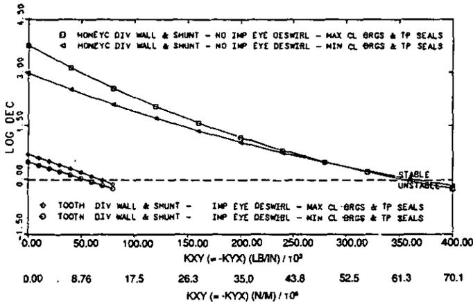
Fig. 9 - Log Dec Vs. Aero. Excitation with Laby Honeycomb Division Wall Laby & No Impeller Eye Deswir vs. Toothed Division Wall Laby & Impeller Eye Deswir
