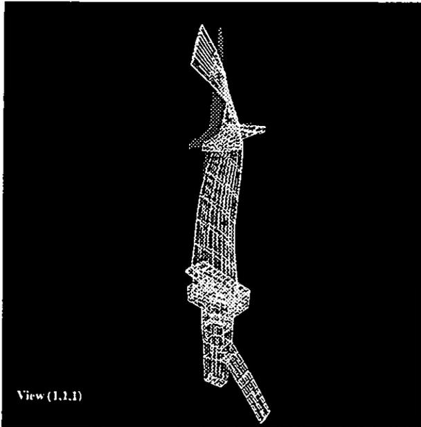
FIGURE 12. Mode 1Ba nodal diameter  $\pm 15$  with BCx.
