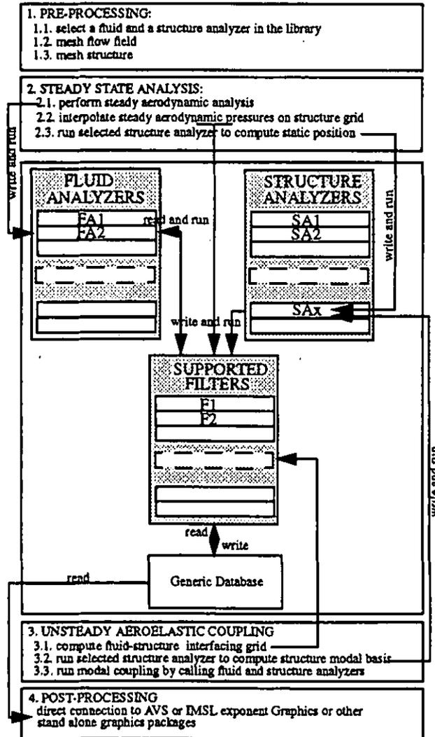
FIGURE 3. Short description of the computer architecture of STRUFLO (Korn Shell program).
