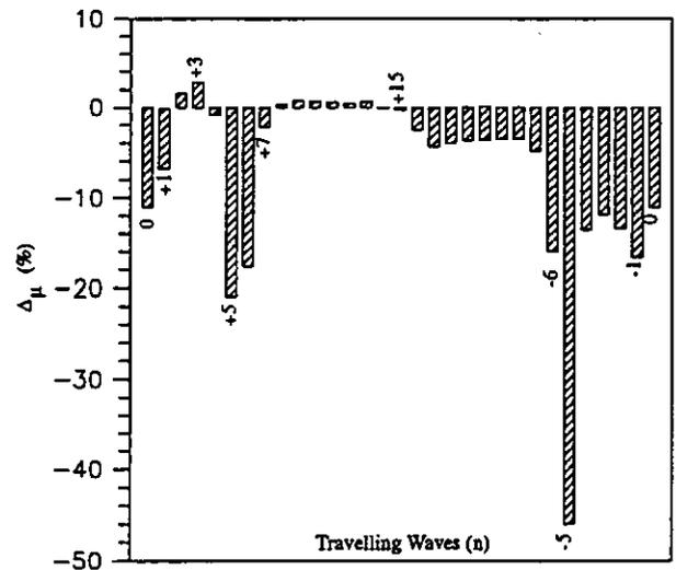
FIGURE 15. Mode 1T, discrepancies for the aeroelastic damping between model BCx and BCxyz, i.e.  $(B_{Cxyz} - B_{Cx})/B_{Cx}$ .
