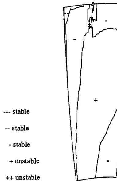
FIGURE 25. MAP contours for mode 1B/-1, model BCx, suction surface.
