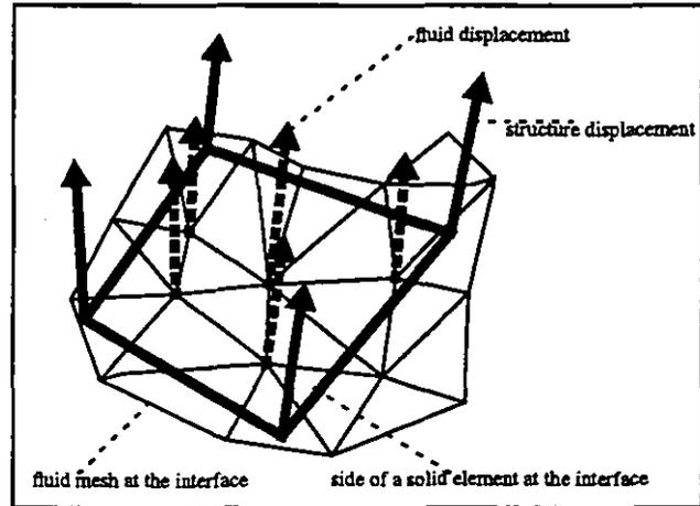
FIGURE 2. Three-dimensional non-matching fluid-structure interface boundary.
