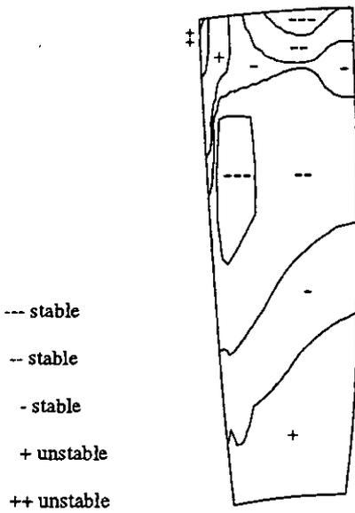
FIGURE 23. MAP contours for mode 1B/-1, model BCx, pressure surface.
