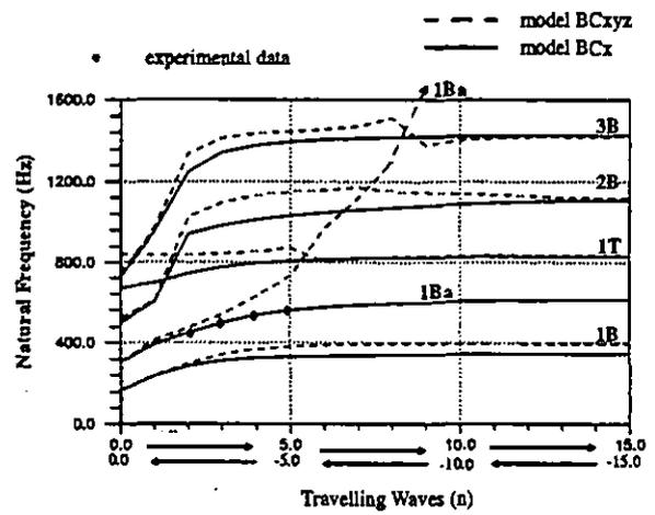
FIGURE 10. Structure natural frequencies as a function of the nodal diameter.
