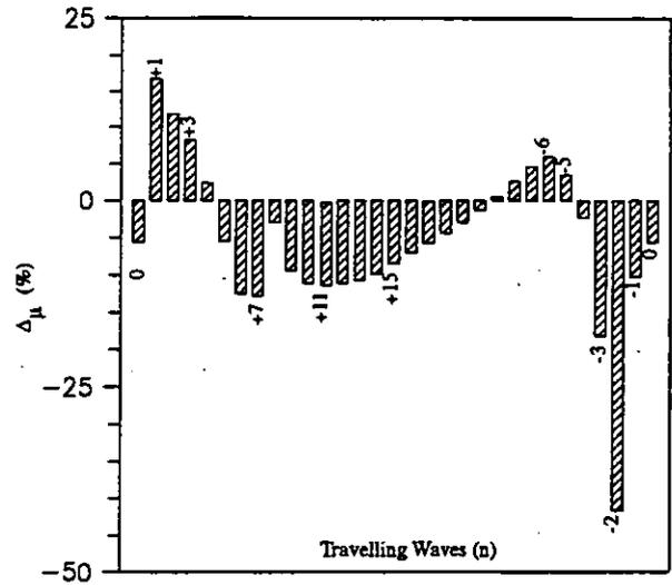
FIGURE 14. Mode 1B, discrepancies for the aeroelastic damping between model BCx and BCxyz, i.e.  $(B_{Cxyz} - B_{Cx})/B_{Cx}$ .
