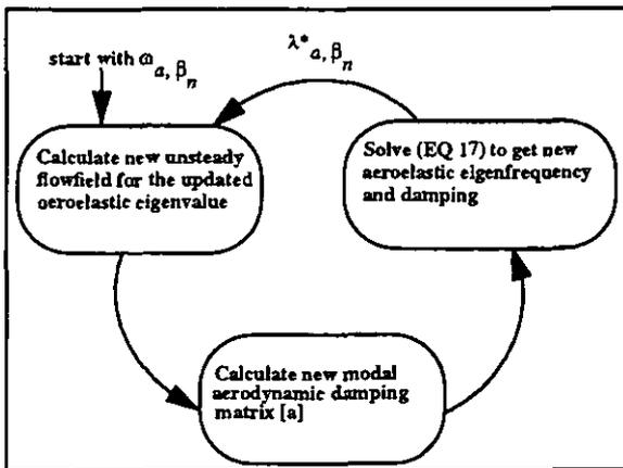
FIGURE 1. Frequency domain aeroelastic iterative procedure.
