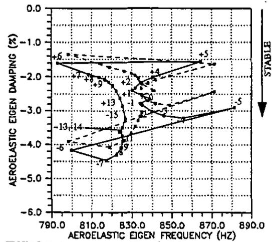
FIGURE 18. Aeroelastic mode 1T, model BCxyz
