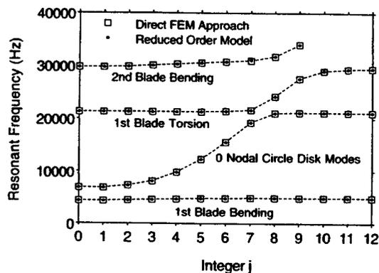
Figure 5: Tuned system frequencies
