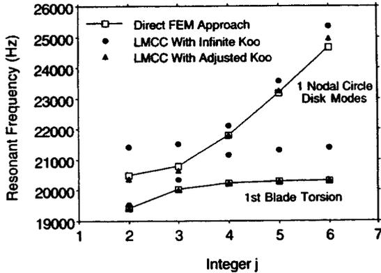
Figure 9: Tuned system frequencies when the disk thickness is reduced by two
