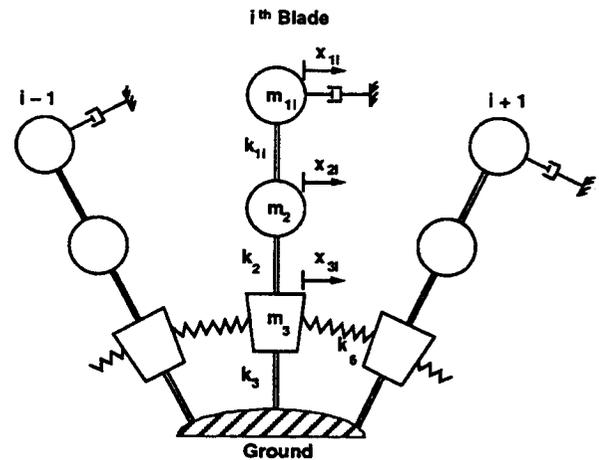
Figure 4: Spring-mass model used by Hoosac and Griffin
