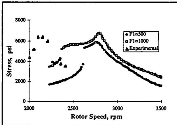
Figure 11: Comparison of Predicted Response with Strain Gage Data
