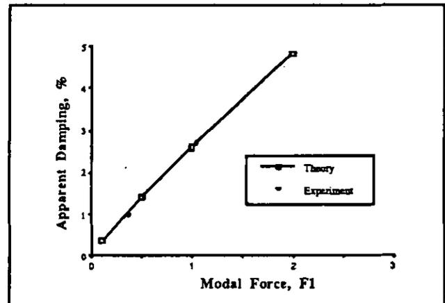
Figure 7: Apparent Damping as a Function of Generalized Force
