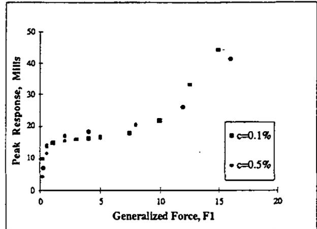
Figure 2: Force Performance Curves for Two Different Values of Baseline Damping
