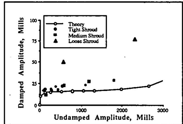
Figure 8: Correlation of Test Data with Predictions
