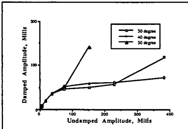
Figure 4: The Effect of Shroud Angle
