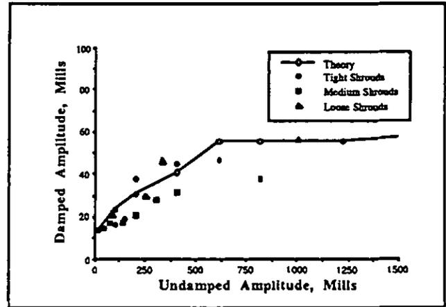
Figure 10: Correlation of Test Data with Predictions
