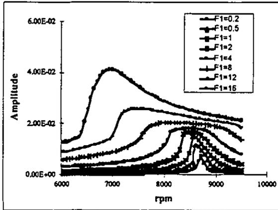
Figure 1: Family of Tracking Plots: Generalized Force Increased From 0.2 to 16.0.
