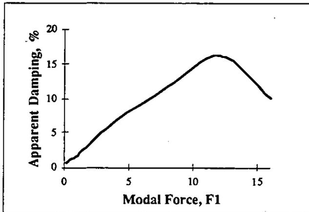
Figure 6: Apparent Damping as a Function of Generalized Force
