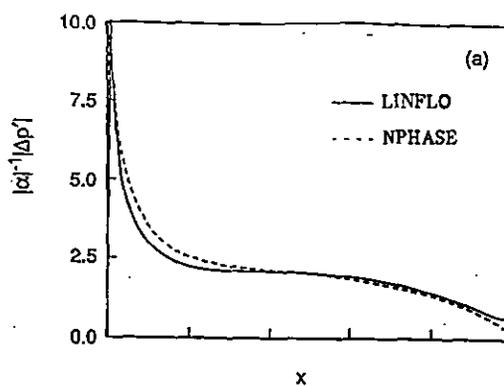
Figure 2: Magnitude of the first harmonic unsteady pressure difference distribution for the Tenth Standard Configuration cascade undergoing an in-phase torsional oscillation of amplitude  $\alpha=2^\circ$  at  $k_1 = 0.5$  about midchord.  $M_\infty = 0.7$ ,  $\Omega_\infty = 55^\circ$ .
