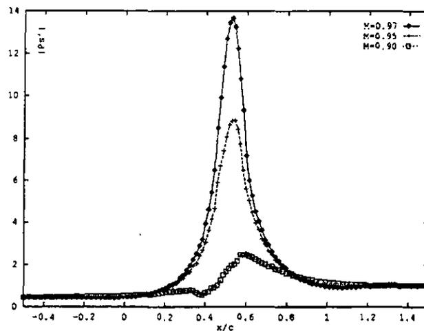
Figure 13: Magnitude of the unsteady pressure distribution for three cross-section locations for the subsonic nozzle case at  $k_1 = 0.3$
