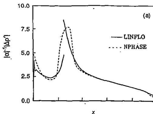
Figure 3: Magnitude of the first harmonic unsteady pressure distribution for the Tenth Standard Configuration cascade undergoing an in-phase torsional oscillation of amplitude  $\alpha=2^\circ$  at  $k_1 = 0.5$  about midchord,  $M_\infty = 0.8$ ,  $\Omega_\infty = 58^\circ$
