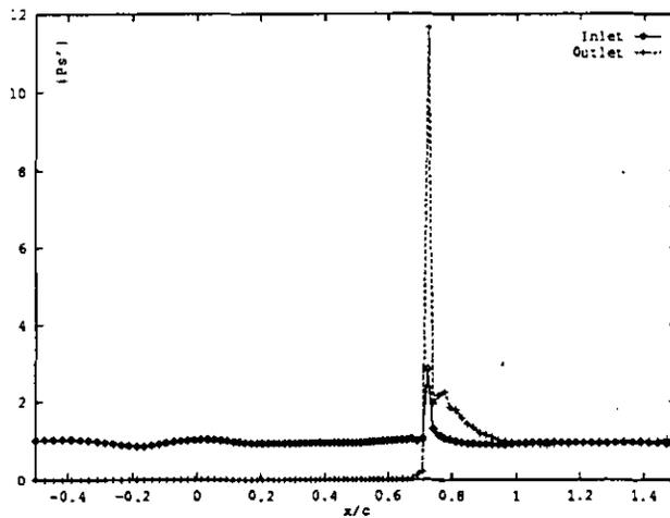
Figure 15: Magnitude of the unsteady pressure distribution along the nozzle surface for inlet and outlet disturbances for the transonic nozzle case at  $k_1 = 0.3$
