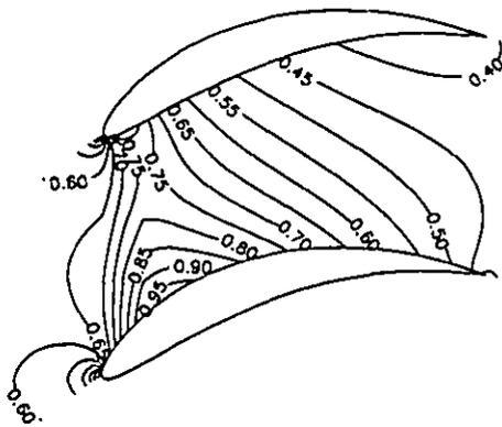
Figure 5: Cascade geometry and the Mean flow Mach number contours for case 3
