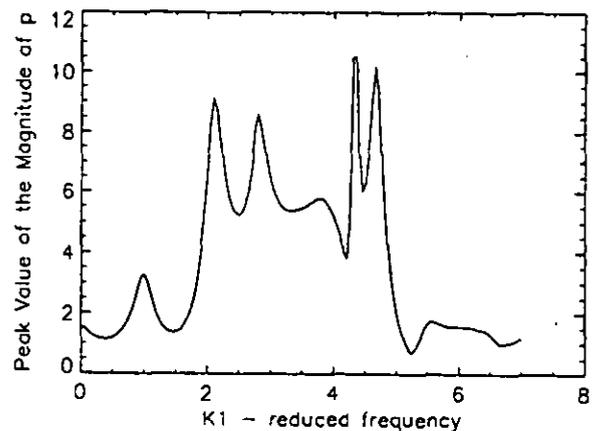
Figure 9: Peak of the magnitude of the unsteady pressure vs.  $k_1$  for case 3 in the region where  $M_{max}$  occurs
