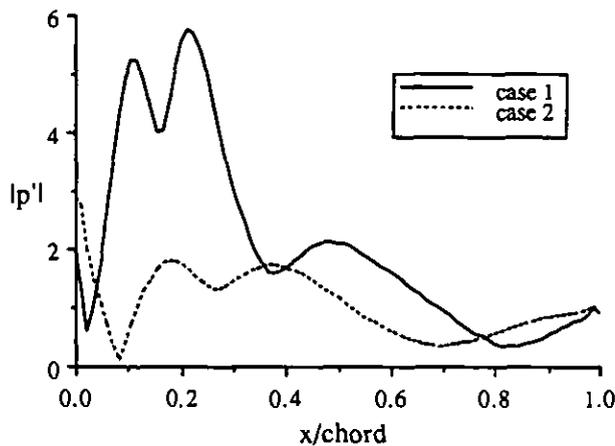
Figure 6: Magnitude of the unsteady pressure distribution along the suction surface of the blade for cases 1 and 2 at  $k_1 = 2.5$
