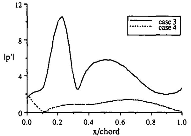
Figure 7: Magnitude of the unsteady pressure distribution along the suction surface of the blade for cases 3 and 4 at  $k_1 = 4.35$
