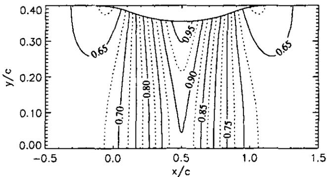
Figure 11: Nozzle geometry and the mean flow Mach number contours for the subsonic case
