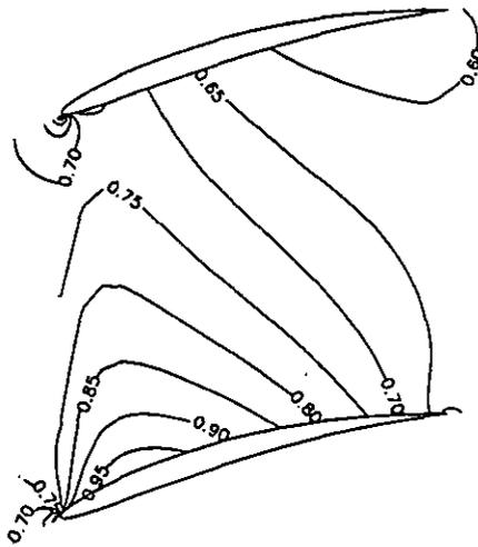
Figure 4: Cascade geometry and the Mean flow Mach number contours for case 1
