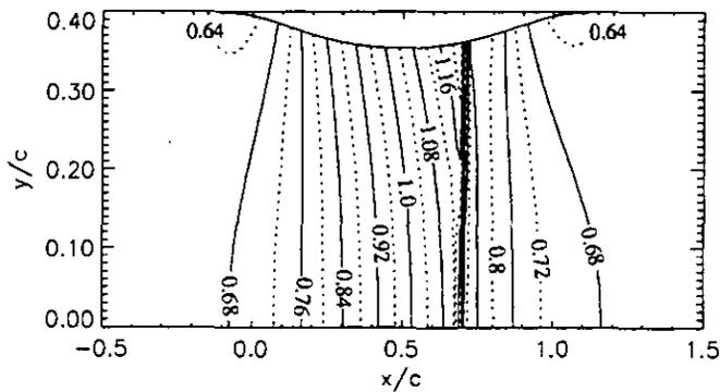
Figure 12: Nozzle geometry and the mean flow Mach number contours for the transonic case
