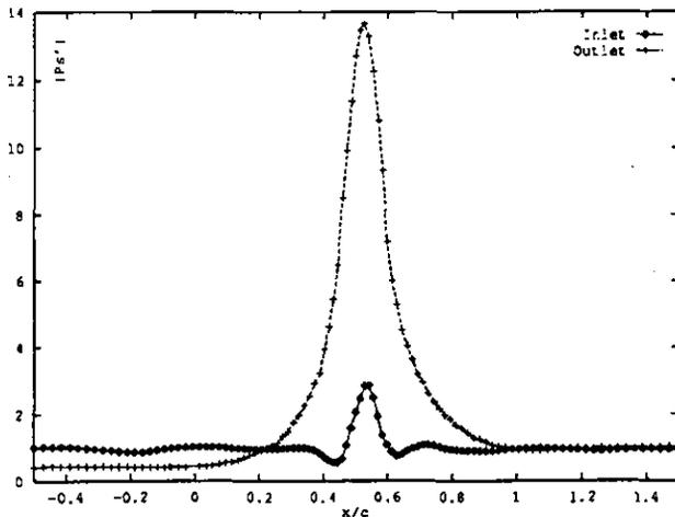
Figure 14: Magnitude of the unsteady pressure distribution along the nozzle surface for inlet and outlet disturbances for the subsonic nozzle case at  $k_1 = 0.3$
