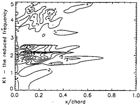
Figure 10: Contours of the magnitude of the unsteady pressure along the blade suction surface vs.  $k_1$  for case 1
