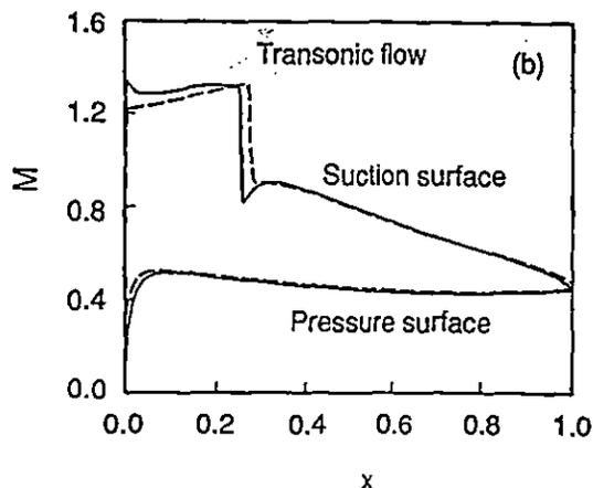
Figure 1: Blade Surface Mach Number Distribution for the Tenth Standard Configuration cascade in transonic flow.  $M_\infty=0.8$ ,  $\Omega_\infty = 58^\circ$
