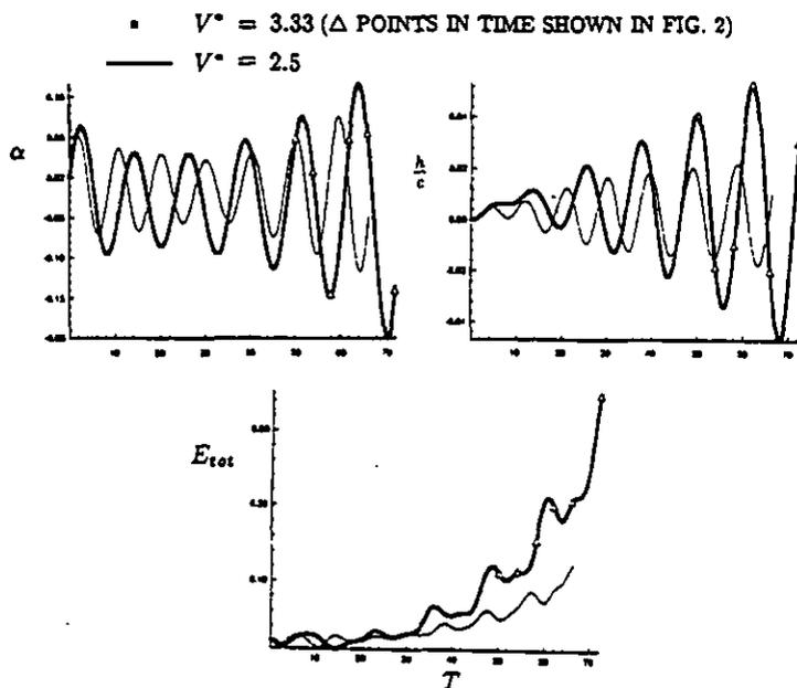
Fig. 3 Histories of  $\alpha$ ,  $\frac{h}{c}$  and  $E_{tot}$  for the unstaggered NACA 0006 cascade with  $\sigma = 180^\circ$  in transonic stall flutter calculations.
