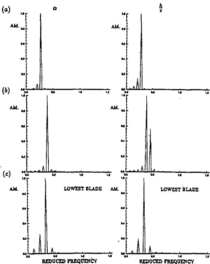
Fig. 9 Fast Fourier Transformation of blade displacements ( $\alpha$  and  $\frac{h}{c}$ ) in transonic choke flutter calculations: (a) cascade with  $\sigma = 180^\circ$  at  $V^* = 3.33$ , (b) cascade with  $\sigma = 180^\circ$  at  $V^* = 2.5$  and (c) cascade with four blades at  $V^* = 3.33$ .
