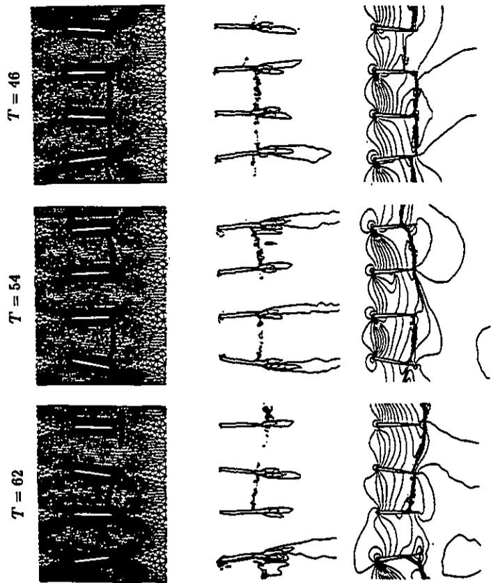
Fig. 10 The sequence of (a) instantaneous meshes, (b) vorticity contours and (c) pressure contours at different points in time for unstaggered NACA 0006 cascade with four blades in transonic choke flutter calculations at  $V^* = 3.33$ .
