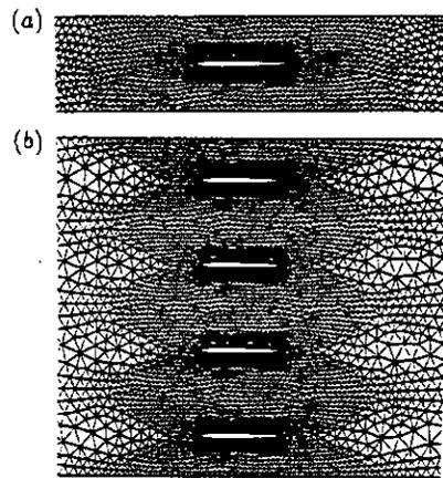
Fig. 1 Coarse meshes (background grids) in transonic stall and choke flutter calculations : (a) NACA 0006 cascade with  $\sigma = 180^\circ$  (4810 elements) and (b) NACA 0006 cascade with four blades (16630 elements).
