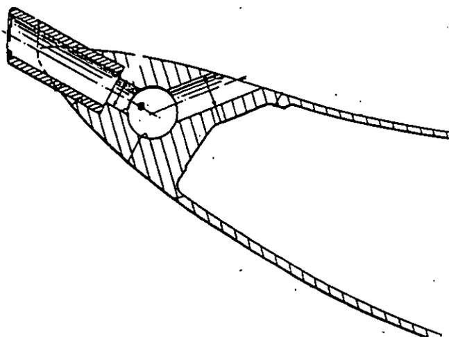
**FIGURE 3: Scarfed Kiel-Shroud for NGV Leading Edge Temperature Sensor, taken from Kokoszka and Tommasini (1985)**
