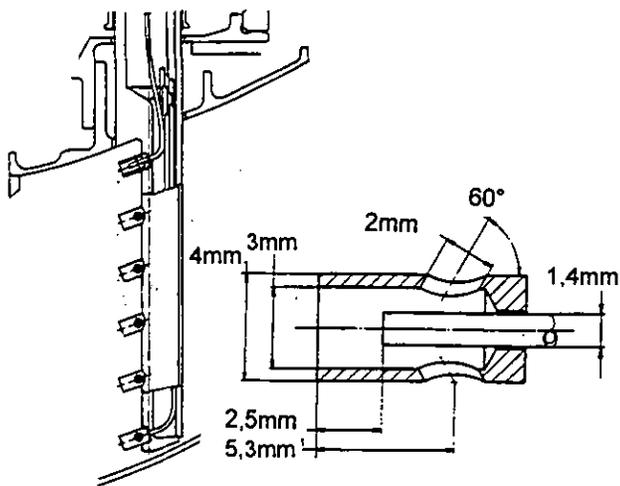
FIGURE 1a): 'Standard' Kiel-Shrouded Pressure Rake Design, taken from Saravanamuttoo (1990)
