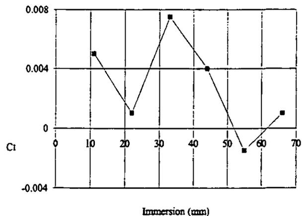
FIGURE 11: Difference in  $C_t$  Values Between Reference and CCR Rakes in Total Pressure Gradient at 0.3 Mn
