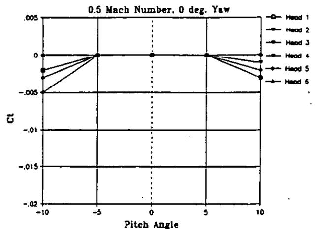
FIGURE 9:  $C_t$  vs. Pitch Angle for Prototype Common Cavity Pressure Rake
