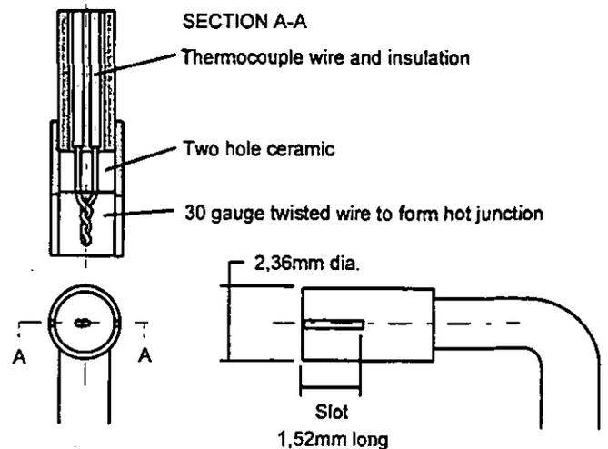
FIGURE 2: Early Kiel-Shrouded Temperature Sensor, taken from Stickney (1955)
