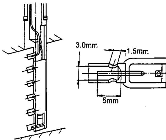
FIGURE 1b): 'Standard' Kiel-Shrouded Temperature Rake Design, taken from Saravanamuttoo (1990)
