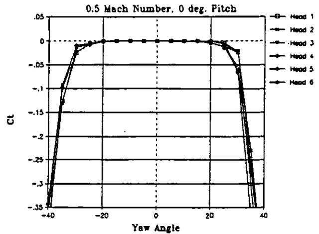
FIGURE 8:  $C_t$  vs. Yaw Angle for Prototype Common Cavity Pressure Rake
