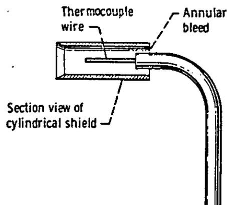
**FIGURE 4: Temperature Probe with Annular Shrouded Thermocouple, taken from Glawe et al.(1978)**
