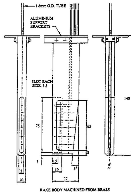
FIGURE 6: Common Cavity Kiel Rake
