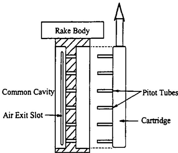
FIGURE 7: Schematic Representation of Pressure Rake Cartridge
