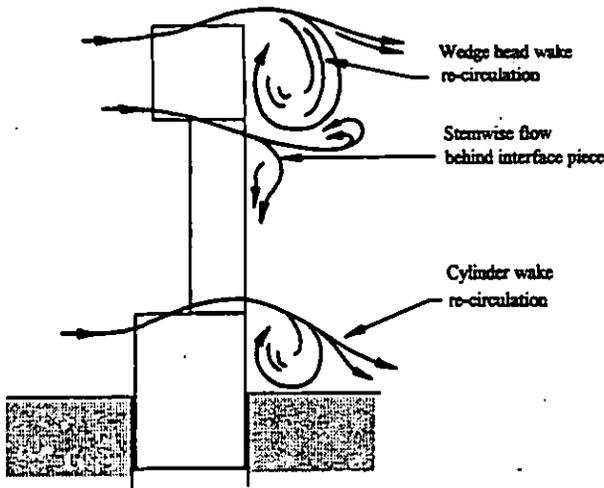
**FIGURE 11: Sketch of 3-D Flow Vis. Results: Probe at 4d Immersion**
