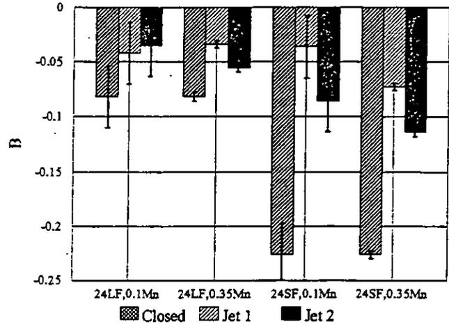
FIGURE 6: Comparison Between B Values for 24° Probes in Open and Closed Flows
