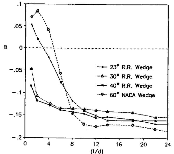
FIGURE 2: Wedge Probe Wall Proximity Effect (Cook, 1988)
