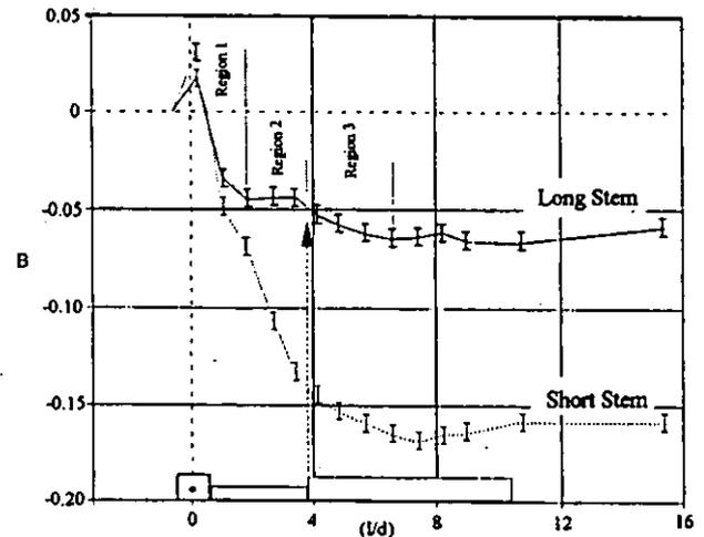
FIGURE 3: Influence of Interface Piece Length on Wall Proximity Effect
