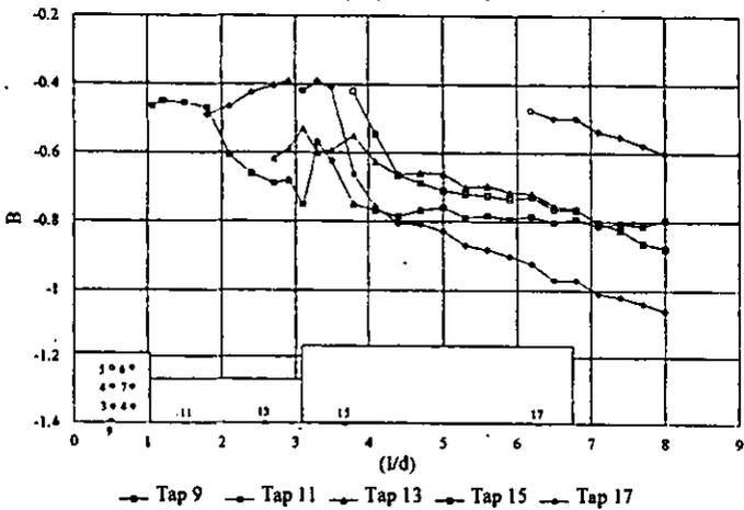
FIGURE 9: Large Scale Wedge Probe Radial Traverse at 25m/s, (taps 9 to 17)
