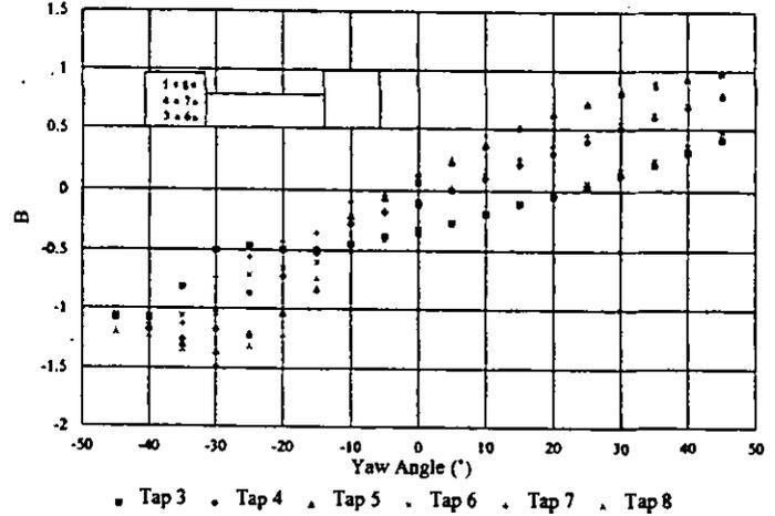
FIGURE 10: Large Scale Wedge Probe Calibration Against Yaw Angle at 25m/s
