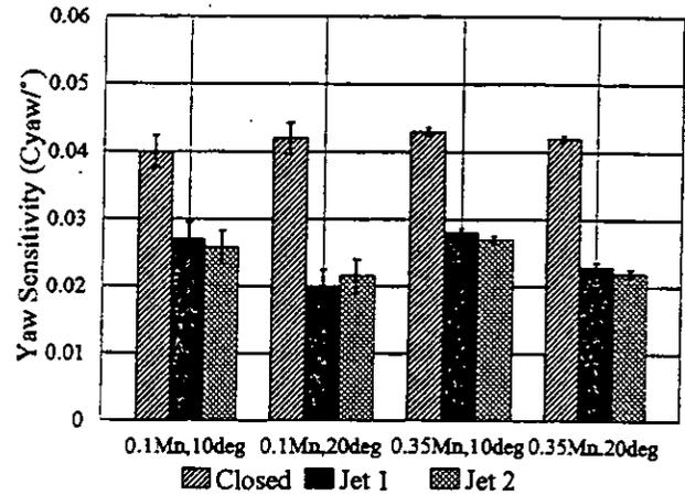
FIGURE 5: Comparison Between Yaw Sensitivities of Short, 24° Probe in Open and Closed Flows
