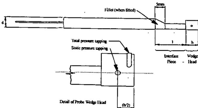
FIGURE 1: Wedge Type Pneumatic Pressure Probe
