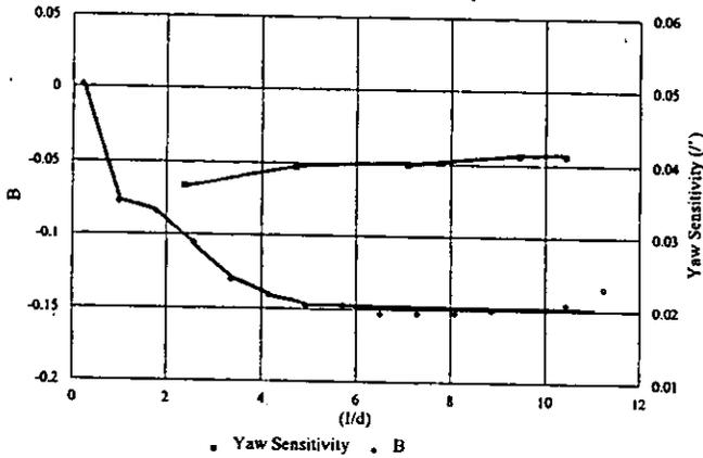
FIGURE 4: 30° Wedge Probe Calibration Against Immersion at 0.1Mn
