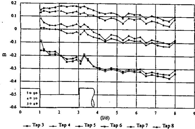
FIGURE 8: Large Scale Wedge Probe Radial Traverse at 25m/s, (taps 3 to 8)
