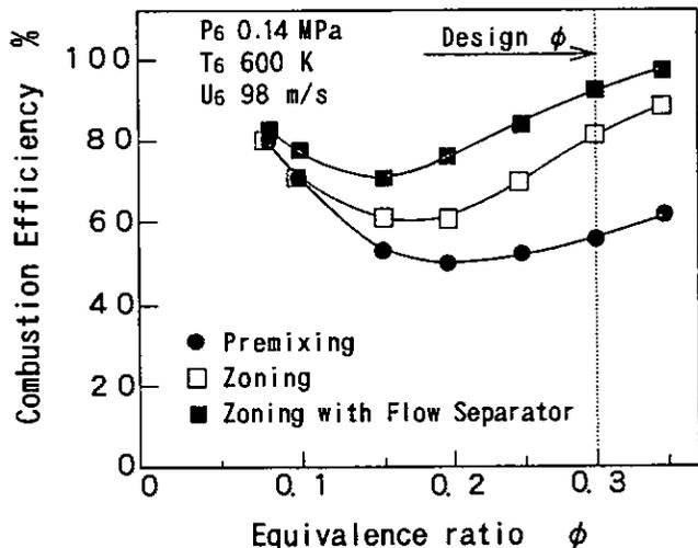
Figure 8 Effect of main fuel nozzle configurations on combustion efficiency
