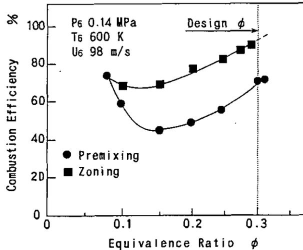
Figure 13 Combustion efficiency of the LSC at Mach 3 condition
