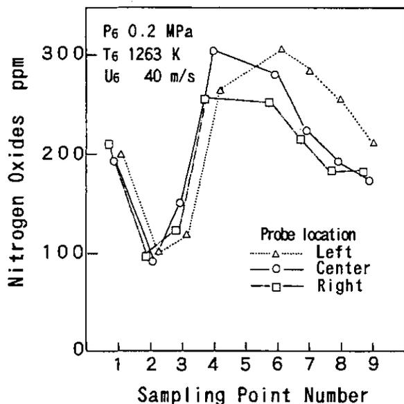
Figure 16 Emission distributions of nitrogen oxides at exit plane
