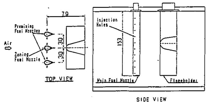
Figure 5 Main fuel injection system and a flameholder of the LSC.
