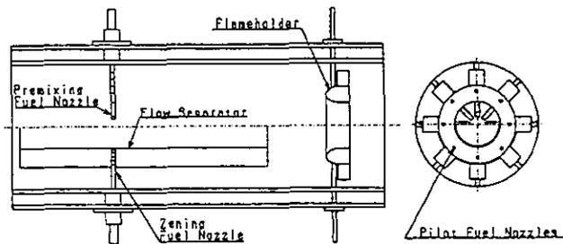
Figure 2 Main fuel injection system and a flameholder of the sub-scale combustor.
