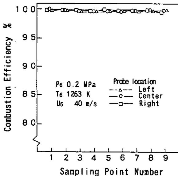
Figure 14 Combustion efficiency at exit plane of the LSC at Mach 5 condition
