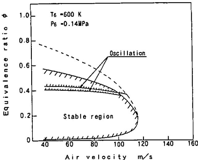
Figure 9 Effect of main fuel nozzle configurations on stability loops
