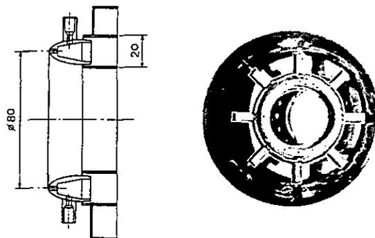
Figure 3 A schematic of the flameholder of the sub-scale combustor.
