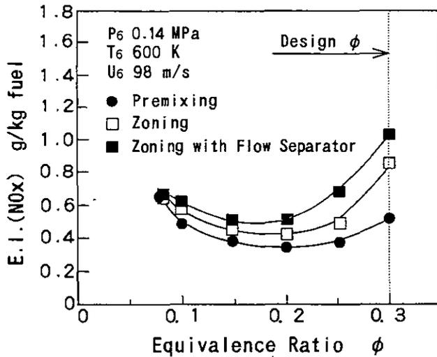
Figure 11 Effect of main fuel nozzle configuration on emissions of nitrogen oxides
