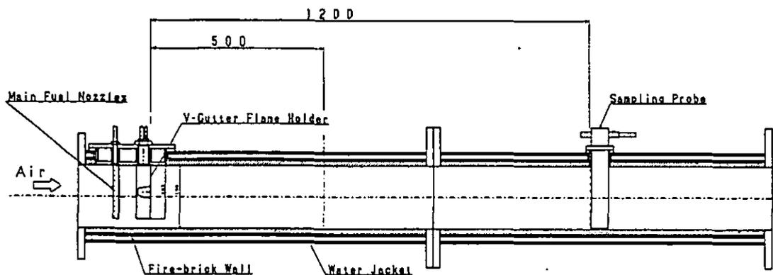
Figure 4 A schematic of the laboratory scale ram combustor.
