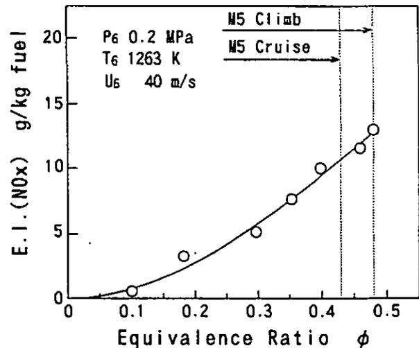
Figure 15 Emissions of nitrogen oxides of the LSC at Mach 5 condition
