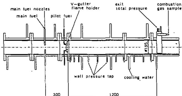
Figure 1 A schematic of a sub-scale combustor for a fuel zoning combustion concept.
