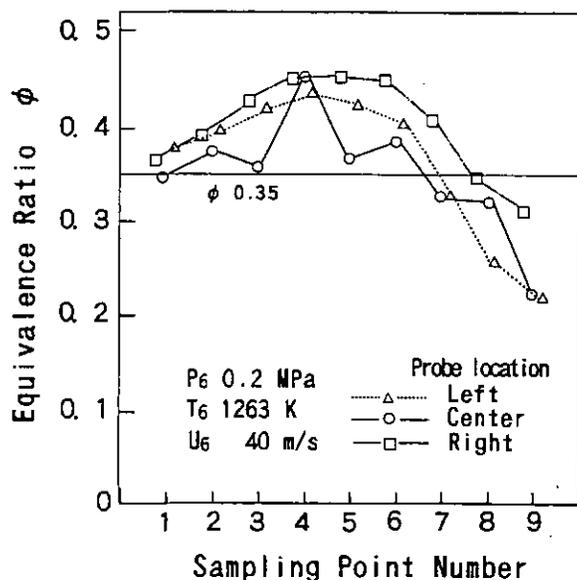
Figure 17 Equivalence ratio distributions at exit plane
