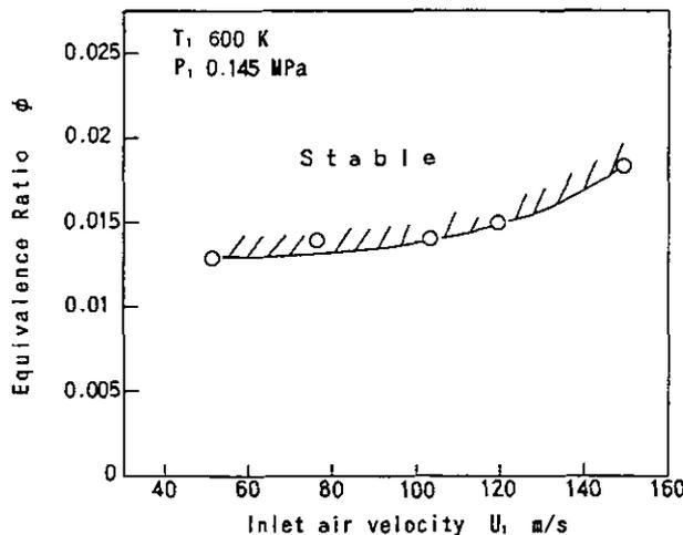
Figure 12 Weak extinction of the LSC at Mach 3 condition
