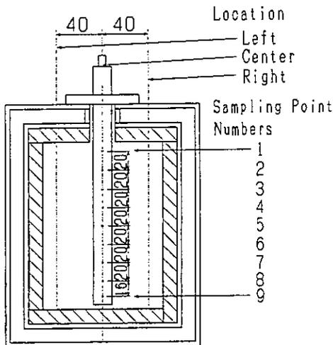
Figure 7 A schematic of sampling points at exit plane.
