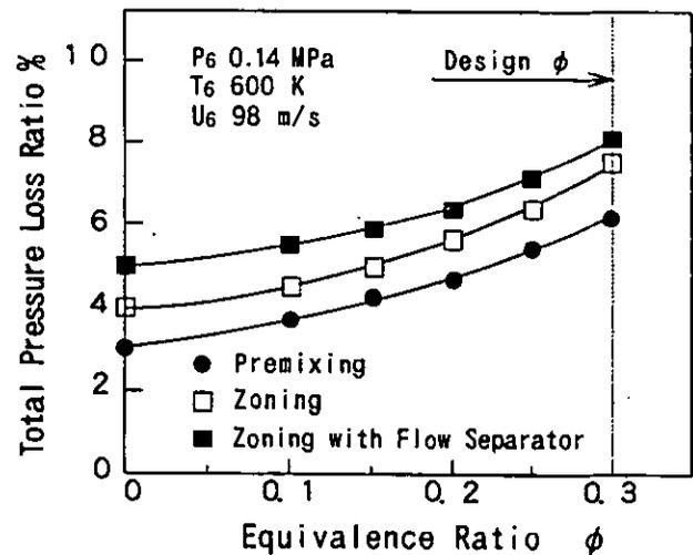
Figure 10 Effect of main fuel nozzle configuration on the total pressure loss ratio
