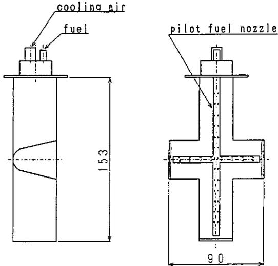
Figure 6 A schematic of the flameholder of the LSC.
