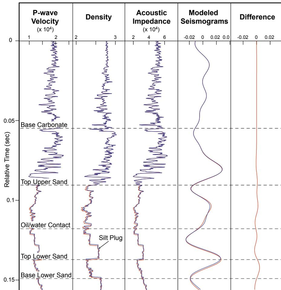
**Figure 5: Modeling results (left to right): P-wave velocity; density; acoustic impedance; modeled seismograms (reverse polarity Ricker wavelet); difference. In the first four tracks, red indicates pay case, and blue indicates wet case. Note, the increase in acoustic impedance below the oil/water contact (OWC) is due to lower porosity due to increased silt content. Just below the OWC, before the facies/lithology change, there is no visually detectable change in impedance (no fluid signature).**
