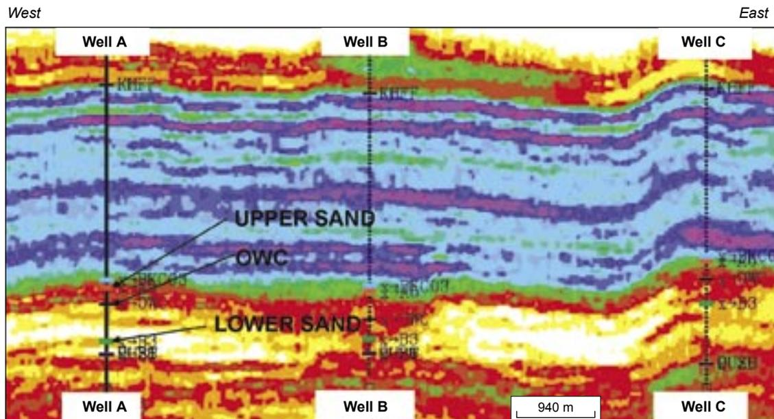
**Figure 3:** Detail of a seismic impedance section passing through three wells. Low impedance (white and yellow) corresponds to good quality of the reservoir. The Upper and Lower Sandstone are, respectively, the Top and the Base of the reservoir.
