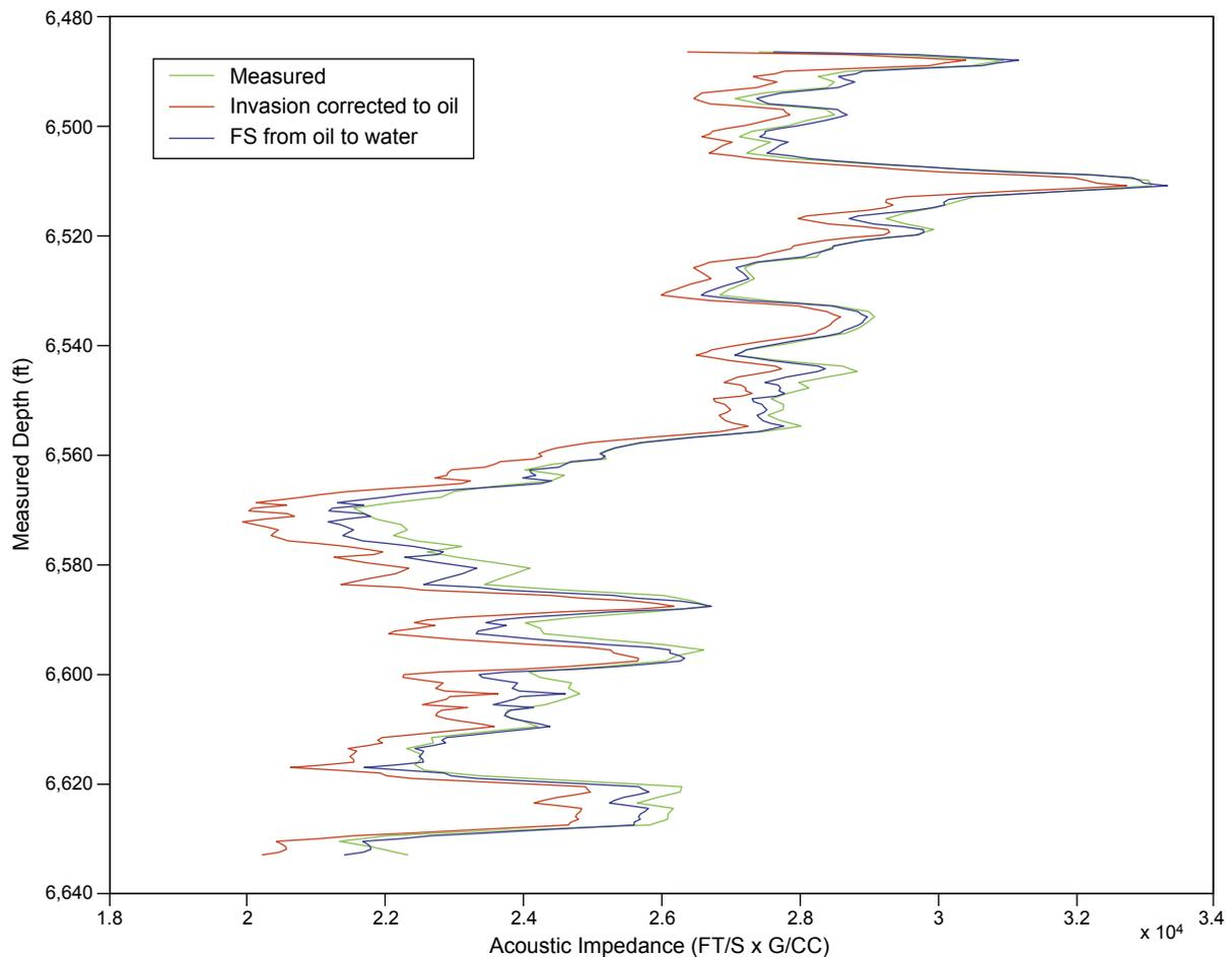
**Figure 4: Fluid substitution analysis in the oil leg of the main reservoir unit, shown for acoustic impedance as a function of measured depth. The oil leg consists of the zone from the top of the upper sand to the OWC.**
