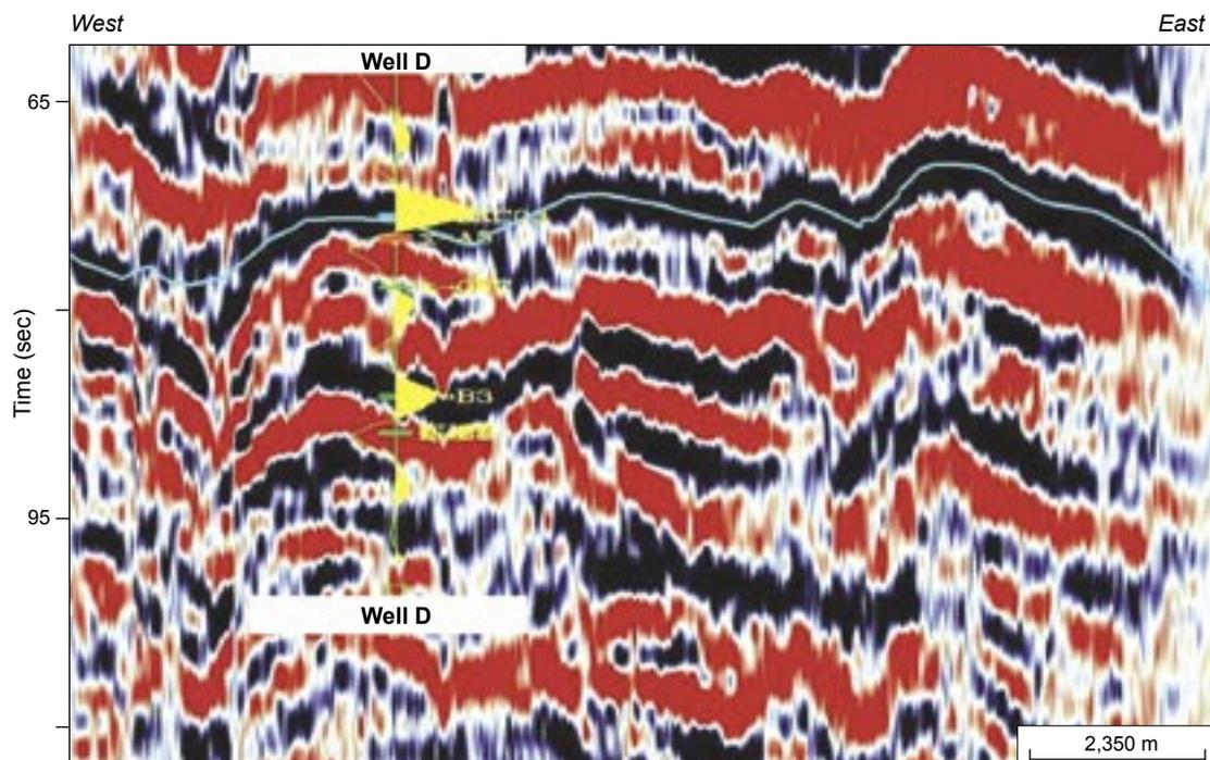
**Figure 2:** Detail of a seismic section at the target. The superimposed yellow trace is the synthetic seismogram estimated from well logs.
