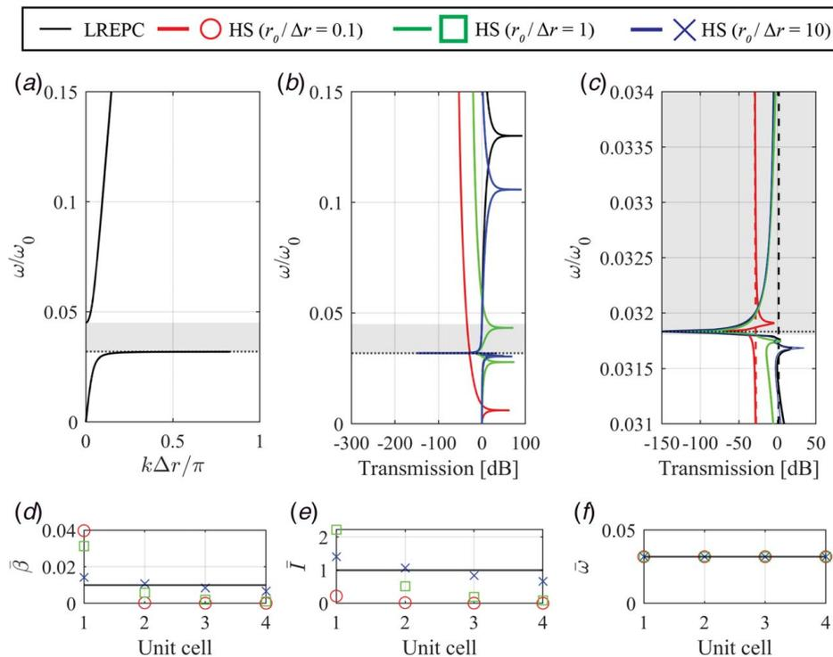
**Fig. 5** (a) LREPC band structure, (b) transmission, (c) zoom in of transmission close to the lower band gap edge, (d)  $\bar{\beta}$ , (e)  $\bar{I}$ , and (f)  $\bar{\omega}$  for each unit cell. Black-dotted lines indicate the resonance frequency of the LREPC and HS resonators. Dashed lines on (c) represent the response of the LREPC and HS system with rigidly attached resonators. For clarity, these are plotted only for the LREPC and the HS with the lower  $r_0/\Delta r$ .
