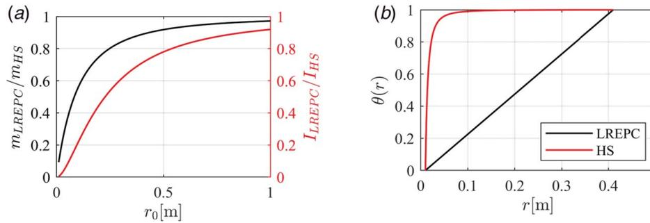
**Fig. 4** (a) Ratios of mass and moment of inertia of four-unit cell LREPC and HS with equal torsional stiffness and (b) static angular displacements of the LREPC and HS with boundary conditions  $\theta(r_0 = 0.01) = 0$  and  $\theta(r_{out} = r_0 + 4\Delta r = 0.41) = 1$
