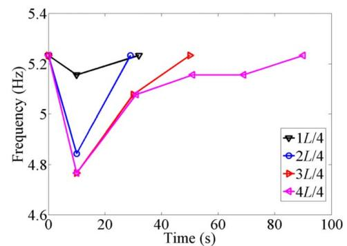
**Fig. 12 Natural frequency variation of the LaSMP laminated beam under mask exposures**
