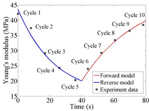
**Fig. 8 Young's moduli data from the chemical kinetics model and the uniaxial tension test (lines: theory; dots: experiment)**
