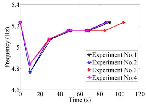
**Fig. 11 Natural frequency variation of LaSMP laminated beam under full UV exposures**
