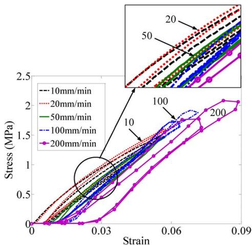
**Fig. 6 LaSMP behaviors under different tension speeds**
