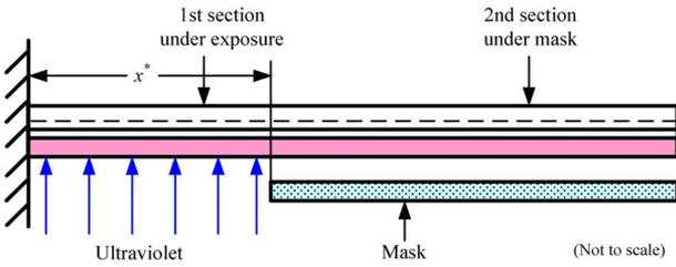
**Fig. 3 The LaSMP laminated beam with mask exposures**
