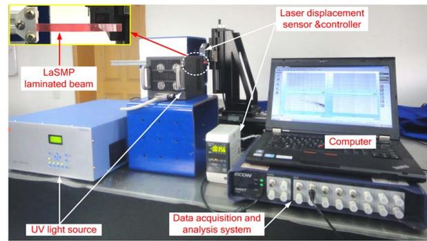
**Fig. 9 Lab setup of the natural frequency control of an LaSMP laminated beam**
