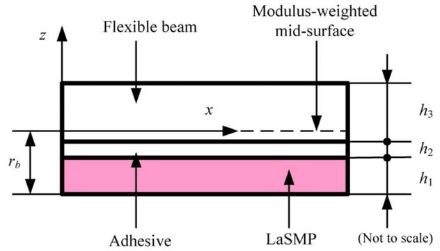
Fig. 2 Cross section of the LaSMP laminated beam
