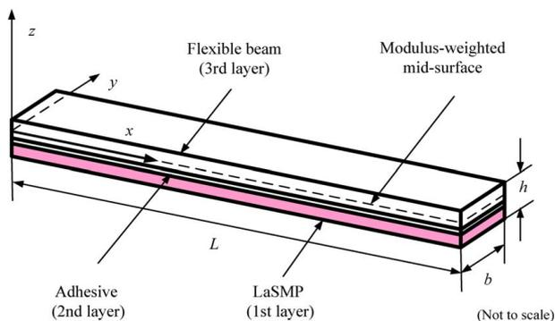
Fig. 1 A three-layer LaSMP laminated flexible beam
