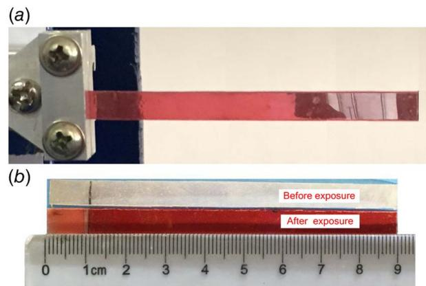
**Fig. 10 LaSMP laminated beam: (a) cantilever beam and (b) beam before and after exposures of UV light**
