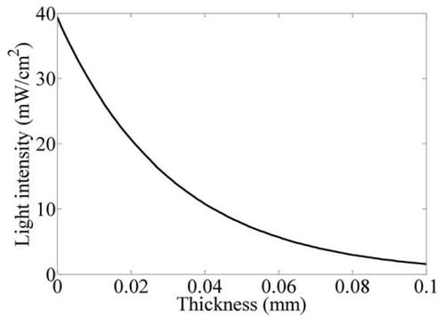
**Fig. 4 Distribution of UV light intensity through the LaSMP sample**
