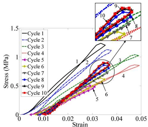
**Fig. 7 Uniaxial tension tests of LaSMP sample (Sp3/EVA\_4)**
