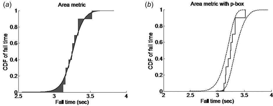
**Fig. 2** Area metrics (shaded in gray) of the same data (helicopter 1 and condition 1 of student A in Appendix B) for different epistemic uncertainty models: a predictive distribution and a p-box of 2.5 and 97.5 percentiles (left and right dashed lines) using  $N$  of 10,000 samples: (a) validation area metric of a predictive distribution (0.032) and (b) validation area metric of a p-box (0.001)
