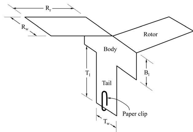
**Fig. 1 Paper helicopter dimensions in meters:  $R_r = 0.1143$ ,  $R_w = 0.0508$ ,  $B_1 = 0.0381$ ,  $T_1 = 0.0508$ ,  $T_w = 0.0254$  (dimensions in inches:  $R_r = 4.5$ ,  $R_w = 2$ ,  $B_1 = 1.5$ ,  $T_1 = 2$ ,  $T_w = 1$ )**
