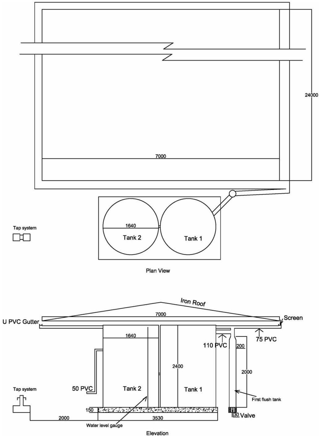
**Figure 2** | Schematic of the RWH system at the Mnyundo Primary School, plan and elevation views, showing the treatment and monitoring components.
