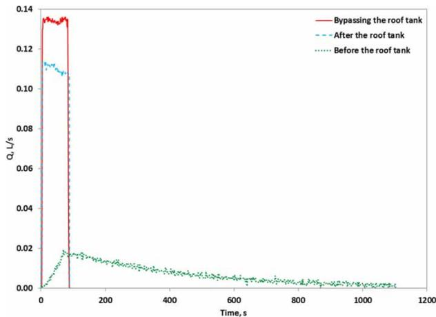
**Figure 9** | The observed flow variation upon activating a common tap, for the three positions of the water meter.
