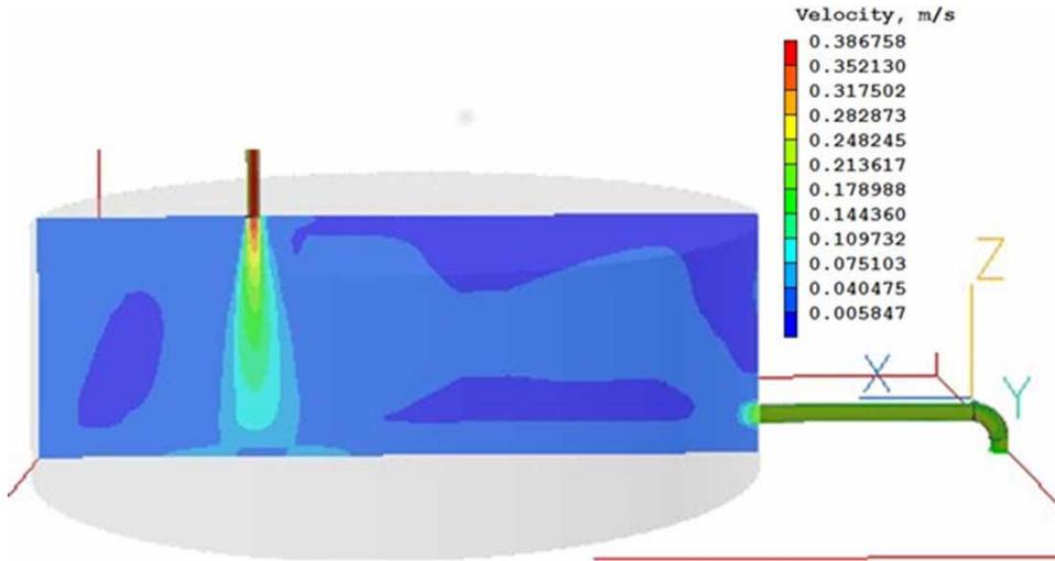
**Figure 6** | The velocity distribution inside the tank obtained by CFD for  $Q=0.10$  L/s and  $V=290$  L.
