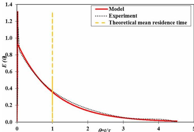
**Figure 5** | The result of the tracer test for  $Q = 0.10$  L/s and  $V = 290$  L, and its three parameter model fitting.
