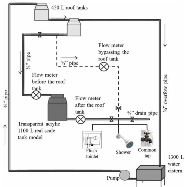
Figure 1 | The experimental setup of the roof tank model.
