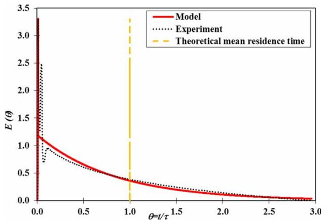
Figure 3 | The result of a tracer test for  $Q = 0.10$  L/s and  $V = 870$  L, and its three parameter model fitting.
