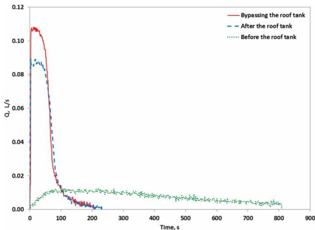
**Figure 7** | The observed flow variation upon activating a flush toilet, for the three positions of the water meter.
