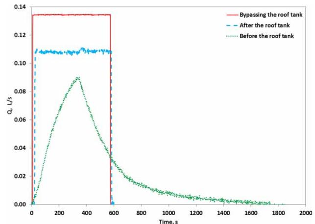
**Figure 8** | The observed flow variation upon activating a shower, for the three positions of the water meter.
