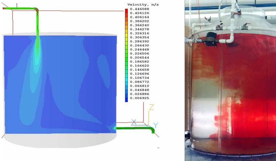
**Figure 4** | The velocity distribution inside the tank obtained by CFD for  $Q = 0.10$  L/s and  $V = 870$  L (left) and the instantaneous colour tracer distribution at time 30 s after the tracer injection (right).
