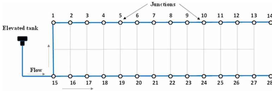
Figure 2 | The distribution network model used for comparing the continuous and intermittent pipe flow.
