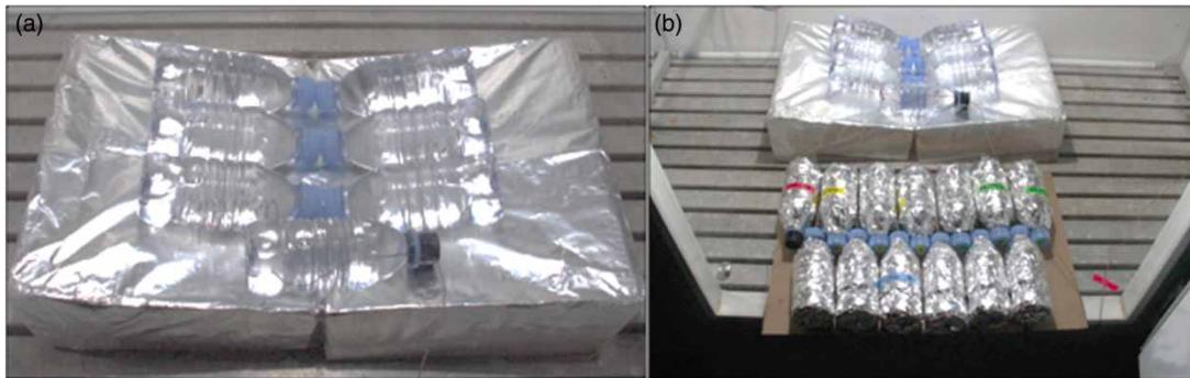
**Figure 4** | SySu disinfection experiment arranged within the controlled chamber. The bottle in the front is the negative control containing a thermocouple (a). Bottles without SySu experiment in foreground were wrapped in tinfoil and placed beneath the bottle stand to ensure no light penetration (b).
