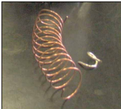
Figure 1 | Copper (64.8 cm) and silver (3.84 cm) wires used for all treatments for water sanitation.
