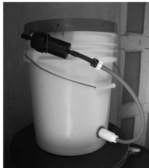
**Figure 1** | Sawyer PointONE™ Filter bucket assembly (secondary storage container not shown).
