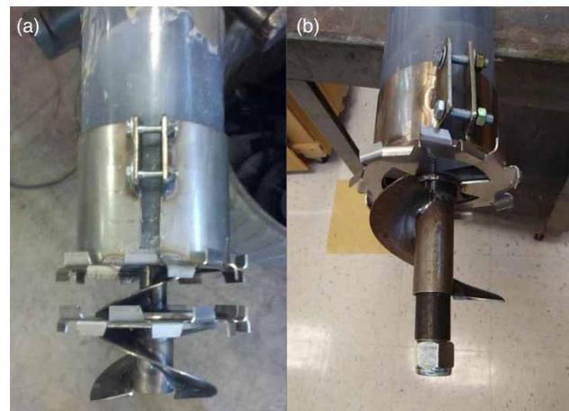
Figure 1 | (a) Double blades and (b) slicer.
