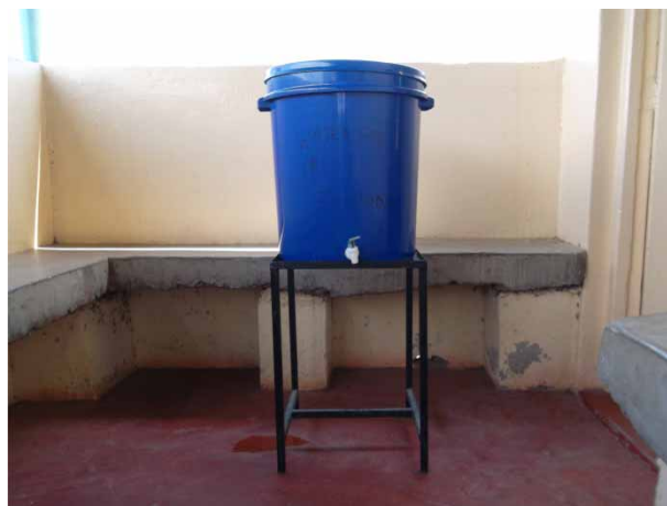
Figure 2 | DWS comprised of a 60-liter bucket with a lid and tap on a simple metal stand.
