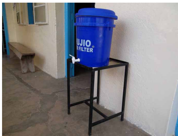
Figure 3 | DWS consisting of a ceramic pot filter (brand name Chujio) nested inside a 60-liter bucket (lid missing from photo).
