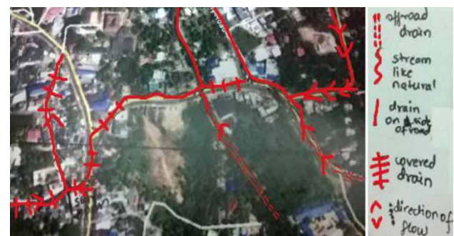
Figure 2 | Sample field data collection map for drainage mapping.
