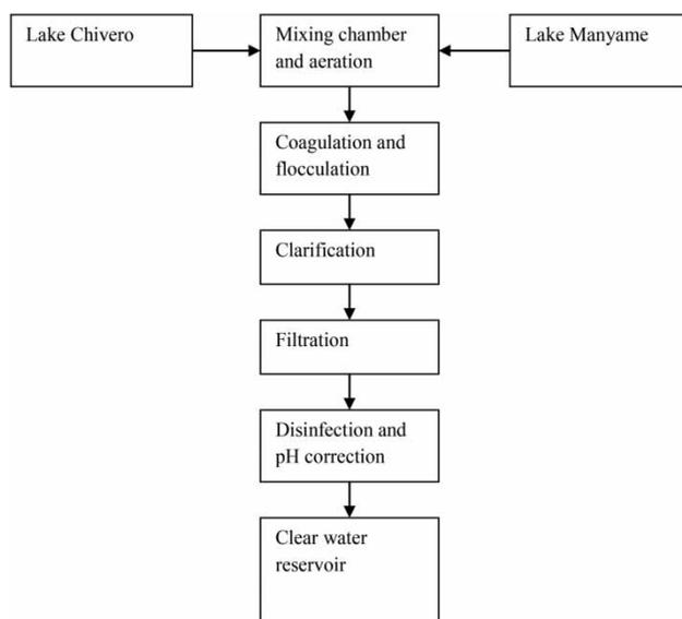
Figure 2 | Flow chart of MJ Water Treatment Works.
