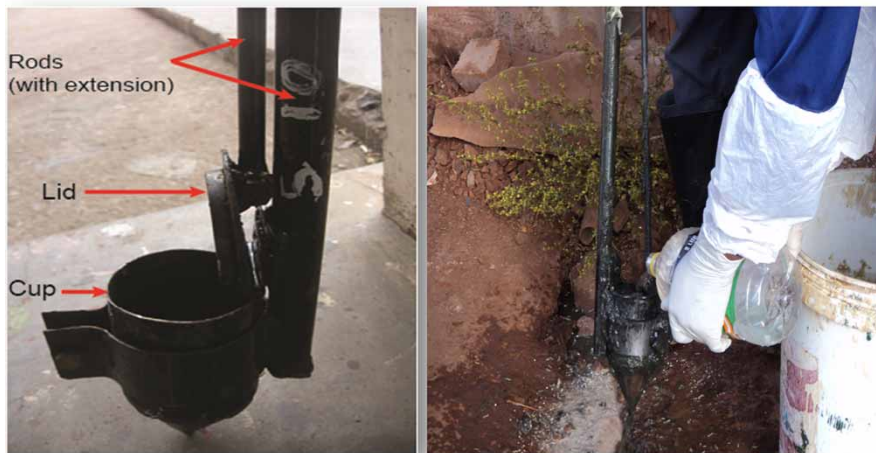
Figure 3 | Modified auger for sampling pit latrine sludge through a squat hole. The modifications made to the conventional auger were the inclusion of a closed conical end, a lid to the cup and a rod to open and close the lid when sampling the sludge from the pit through the squat hole.
