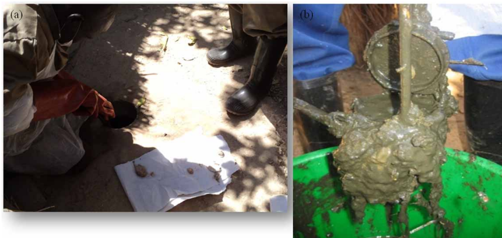
Figure 4 | Pit latrine sludge sampling: (a) collecting sludge from a pit latrine through a squat hole and (b) pit latrine sludge withdrawn from the pit before being put in polythene bottles.
