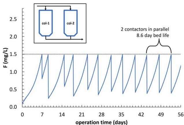
**Figure 3** | Simulated operation of two bonechar contactors ( $EBCT$  38.2 minutes,  $F_{C_0} = 8.5$  mg/L) in staged parallel mode. The polynomial fit to column 1  $F$  breakthrough data (Figure 2(a)) was used to simulate several cycles of operation using MS Excel. The inset shows the treatment flow diagram.
