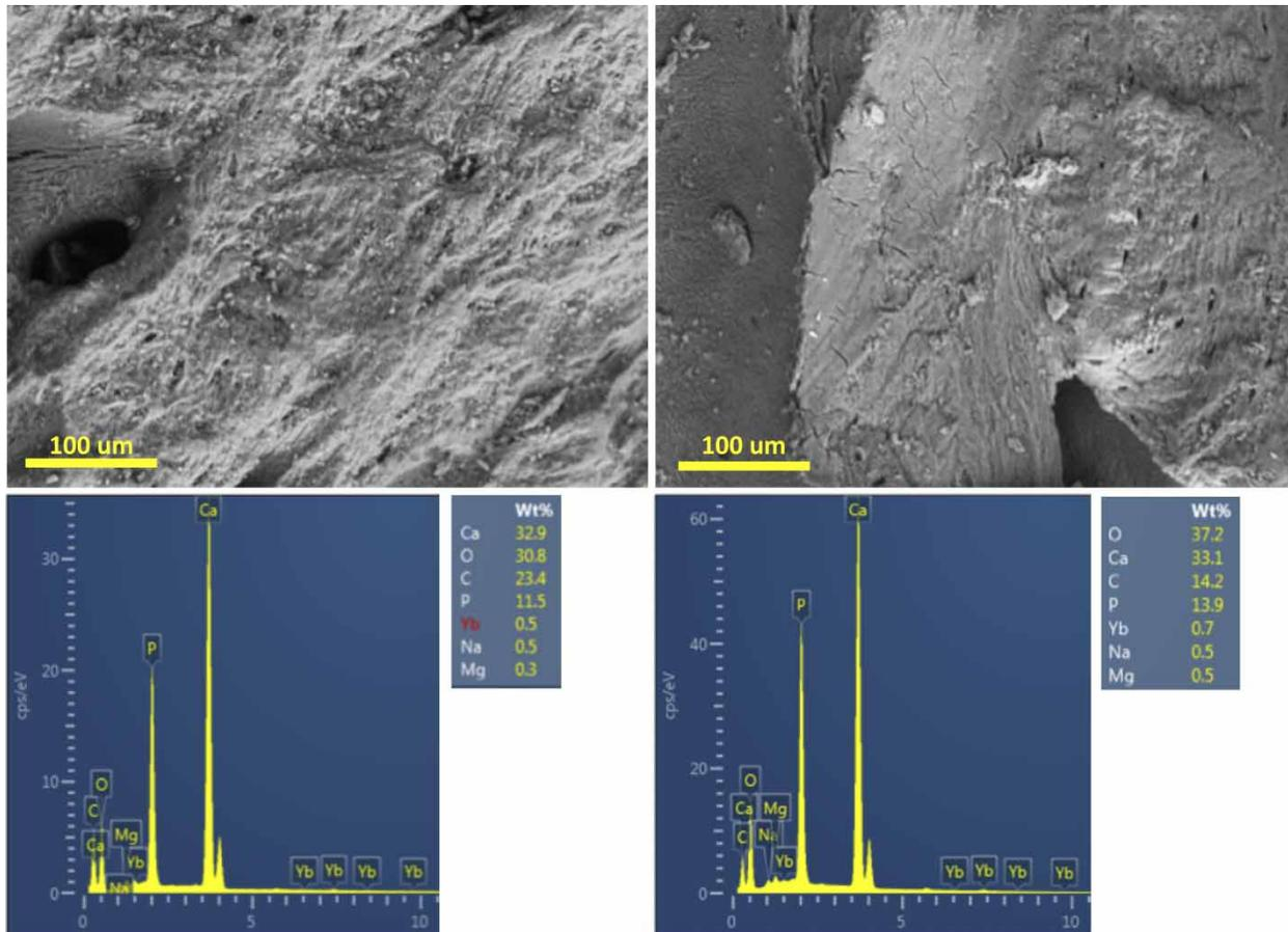
Figure 1 | VP-SEM images and EDS spectra of bonechar granules.
